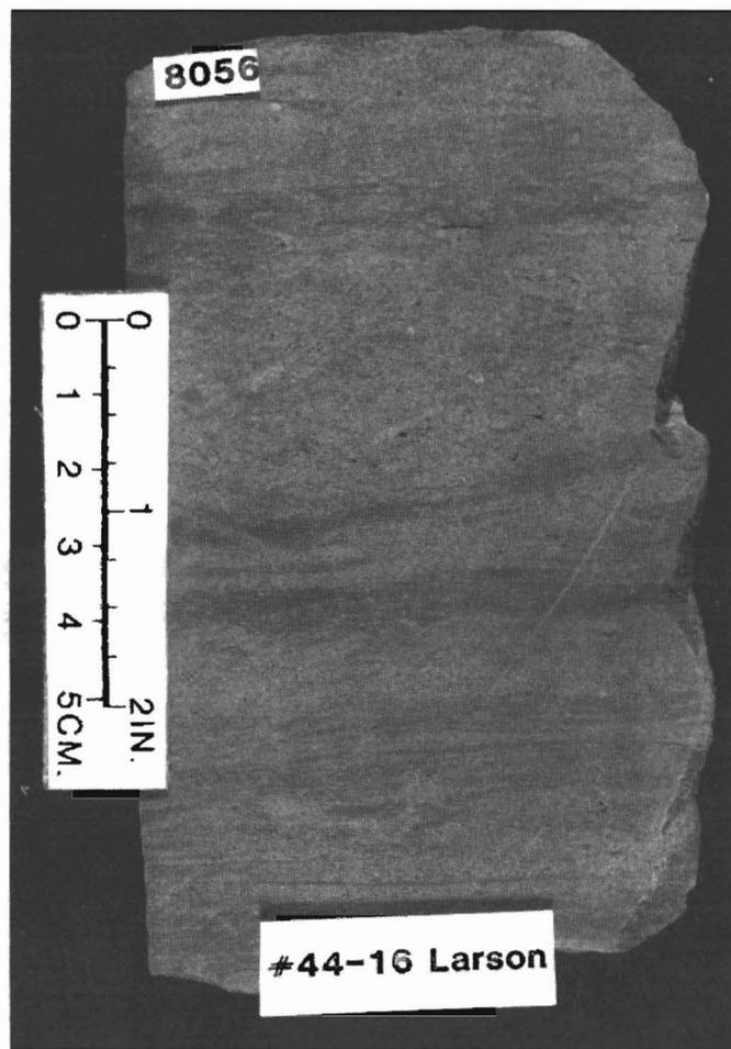
Figure 9b. (Facies 3). Subhorizontal laminations are well preserved at the base of this restricted subtidal sample from the Flat Lake subinterval in the Depco, #44-16 Larson, SESEsec 16, T159N, R102W. Small Chondrites burrow structures and wispy laminations are present in the upper portion of the sample.
