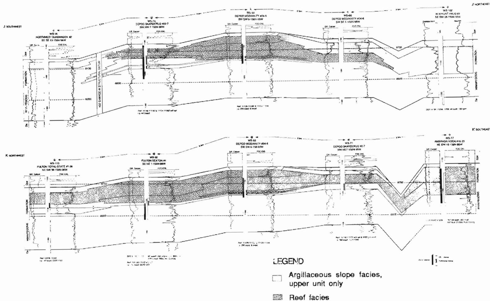
**Fig. 5** - Temple Field structural cross sections J-J' and K-K' (refer to Fig. 4A). Depositional dip section J-J' illustrates stratigraphic relationships of reef and underlying slope reservoir facies. Depositional strike section K-K' illustrates variable reef development along the platform margin. FDC-CNL log cross over in upper portion of most wells indicates salt plugged carbonate. O/W denotes original oil/water contact in the reservoir.
