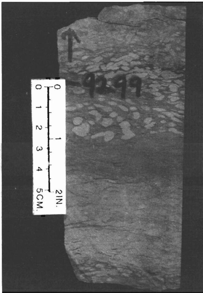
Figure 7a. (Facies 2). Well preserved Chondrites burrow structures from the restricted subtidal facies, Depco-Pennzoil, #22-32 Federal, SWNEsec 22, T147N, R101W.
