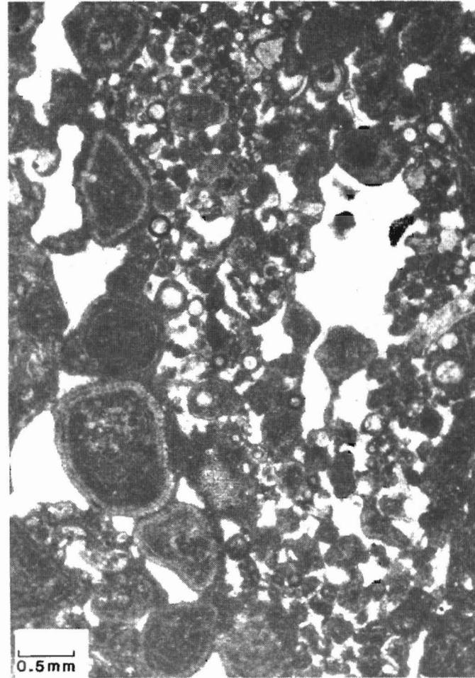
Figure 11b. (Facies 4). Calcispheres, peloids, and coated grains are part of the allochem assemblage in this packstone. Fenestral porosity is occluded with calcite spar and baroque dolomite cements. Intergranular porosity is partially preserved near the top of this photomicrograph. Sample from 9145 feet in the Sun Exploration and Production, #2 Erickson, NWNEsec 27, T152N, R102W.
