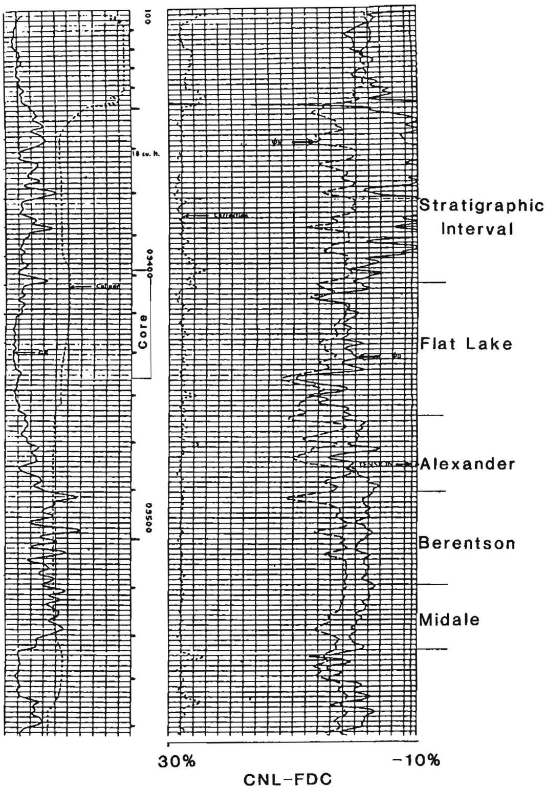
Figure 3. Type log showing the subintervals of the Ratcliffe in the central basin. Production is from the Alexander and Flat Lake intervals.
