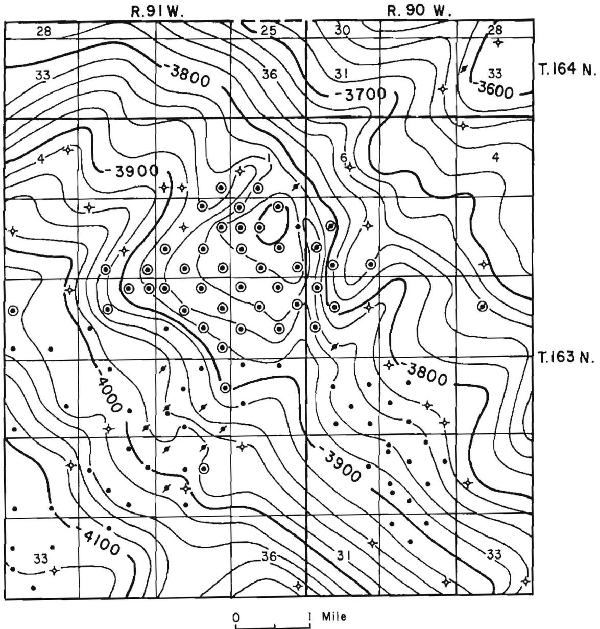
Figure 3. Flaxton field area, Burke County, North Dakota, current interpretation of Mission Canyon structure. 20 ft (6m) contours. Mission Canyon producers are circled; other wells are Midale and/or Nesson completions.
