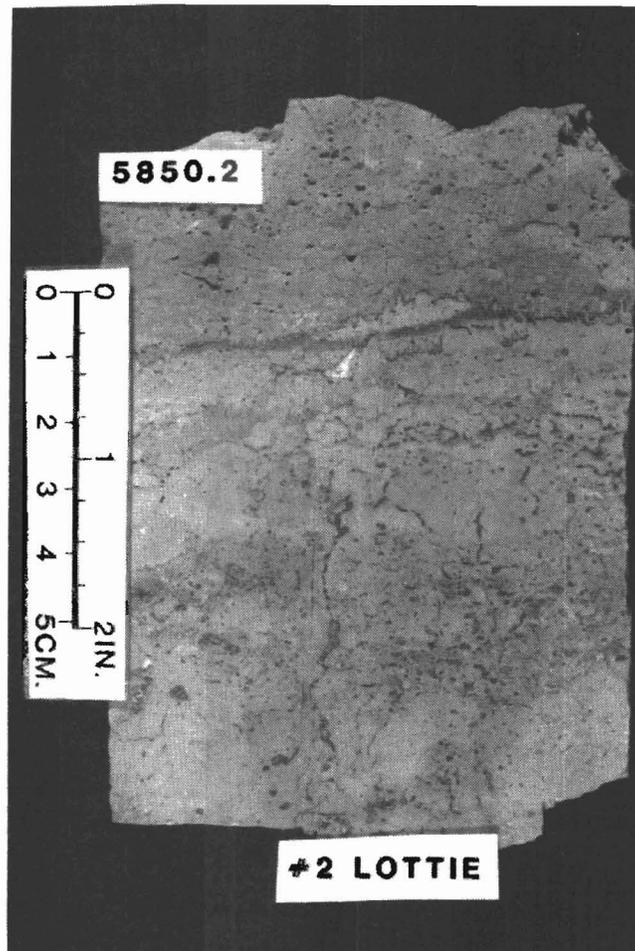
Figure 9. 5850' Ostracod calcisphere wackestone, Coteau interval. Top of main porosity streak in Coteau.
