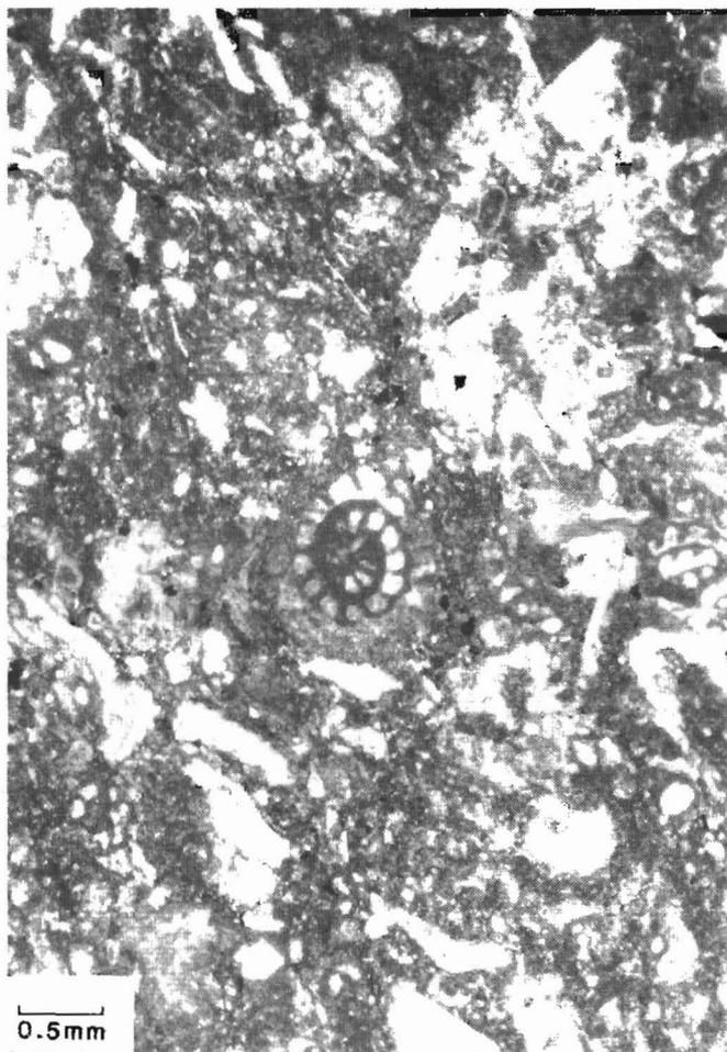
Figure 6c. (Facies 1). An endothyrid foraminifer (center) is surrounded by crinoid, brachiopod, and other skeletal fragments. From 8767 feet in the Arco, #1 State Gafkjen, SESEsec 36, T158N, R100W.
