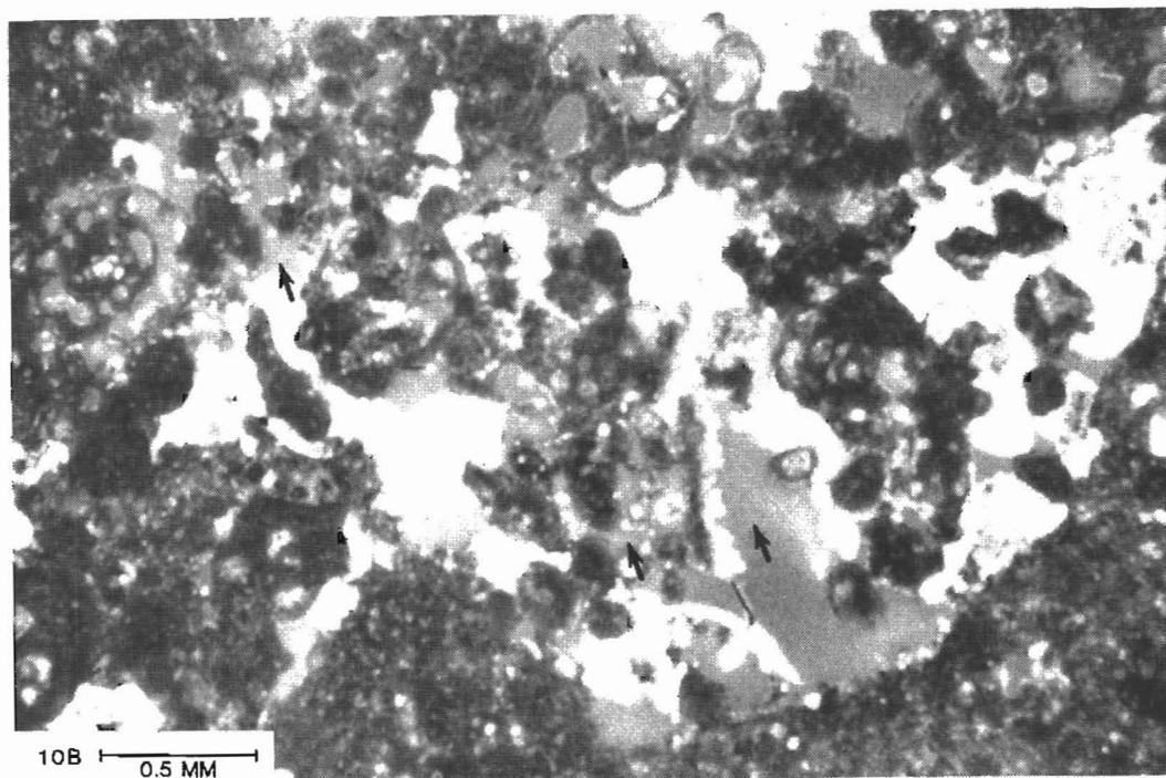
Figure 10. (A) Oolith-pisolith grainstone, 1 Marvin well, SESWsec 12, T163N, R91W, 5777.5 ft. Note drusy calcite lining fenestral pores which are partially to completely infilled with blocky calcite (labelled "C" on photo). (B) Bioclastic packstone and grainstone, 2 Galvin well, NWNWsec 12, T163N, R91W, 5318.5 ft. Note good interparticle porosity.
