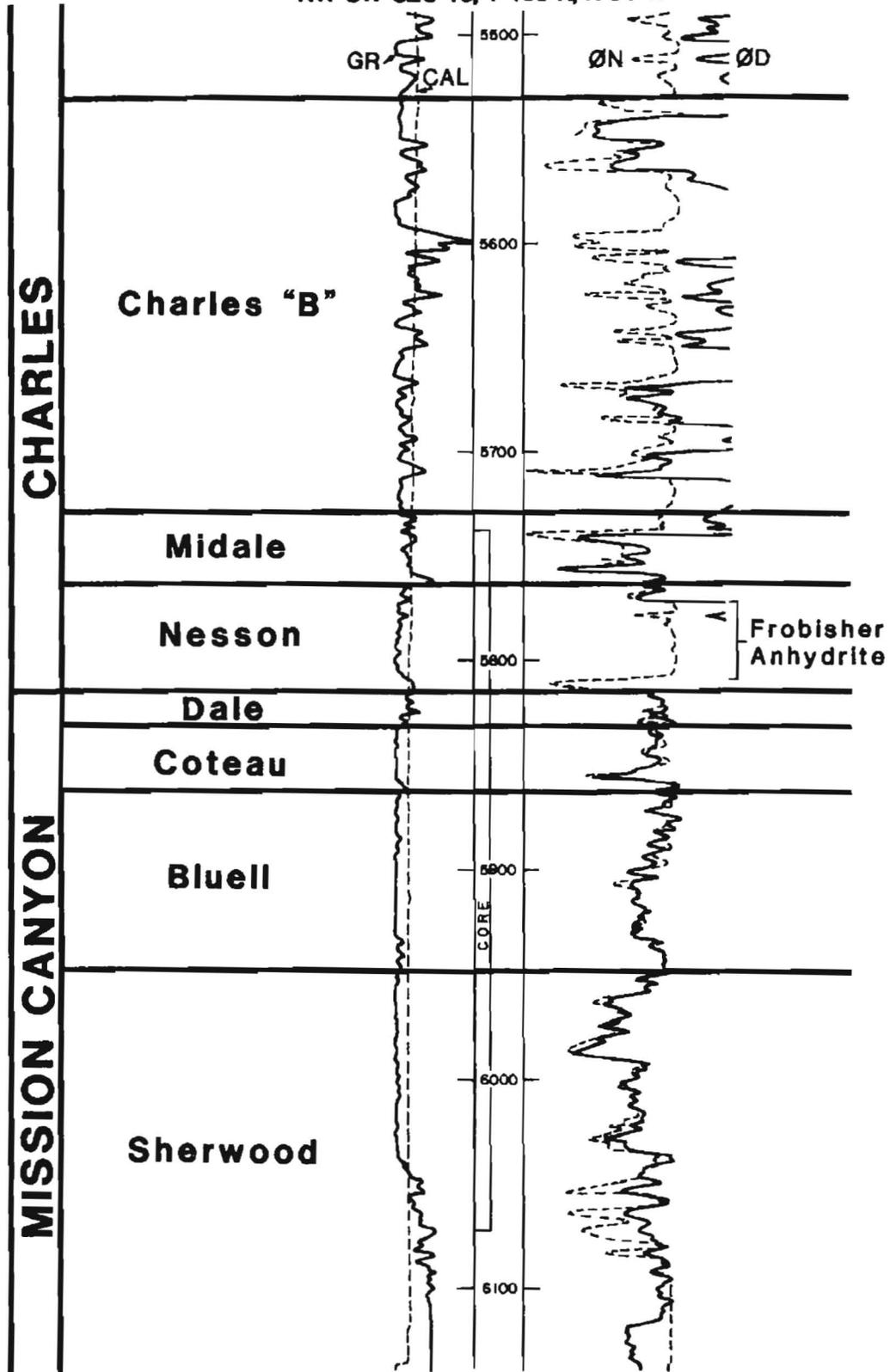
Figure 4. Gamma ray-compensated neutron-formation density log of Monsanto 2 Lottie, NWSwsec13, T163N, R91W.
