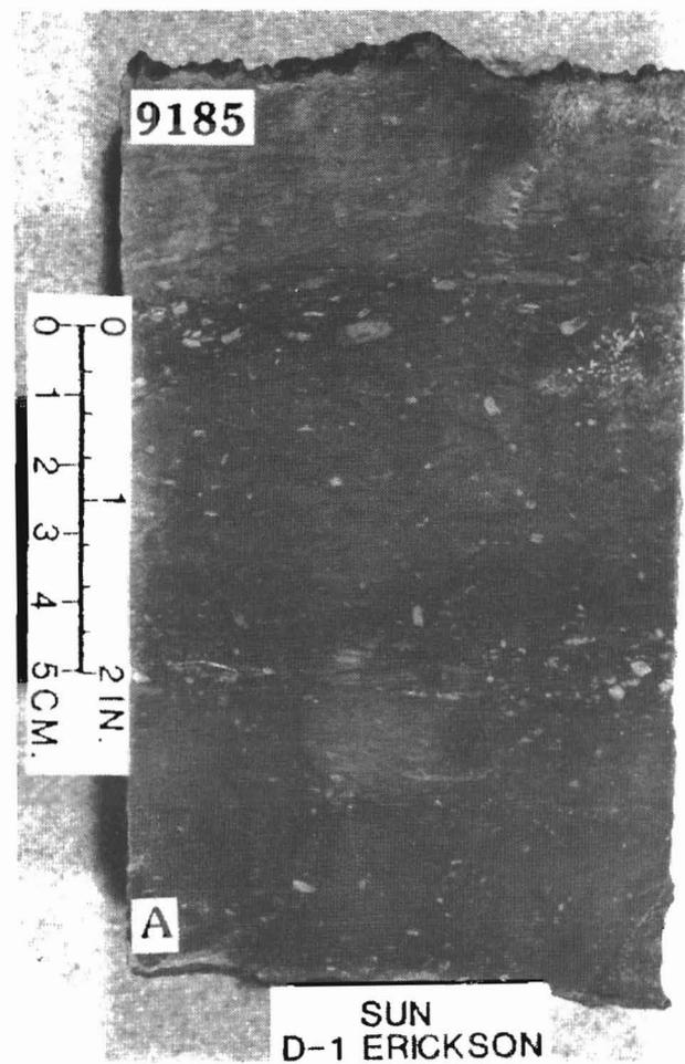
Figure 5d. (Facies 1). A crinoidal wackestone from the shallow shelf facies, Sun Exploration and Production, #1 D. Erickson, SENWsec 27, T152N, R103W.
