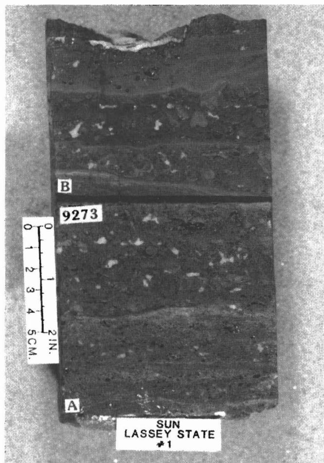
Figure 10c. (Facies 4). A peloidal and coated grain packstone from the Sun Exploration and Production, #1 Lassey State, SWSWsec 28, T152N, R103W, shows thin, shal- lowing upward beds typical of the grain-rich por- tions of the Flat Lake subinterval. The white occluding cements are baroque dolomite and sparse anhydrite. Lack of interconnection has rendered most vuggy pores ineffective.
