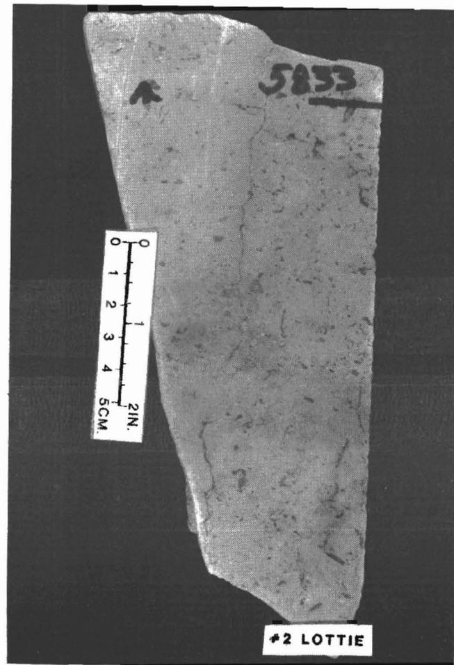
Figure 8. (B) 5833' Mudstone, Coteau interval. Vertical fractures, now mostly cemented, are important contributors to permeability when open.
