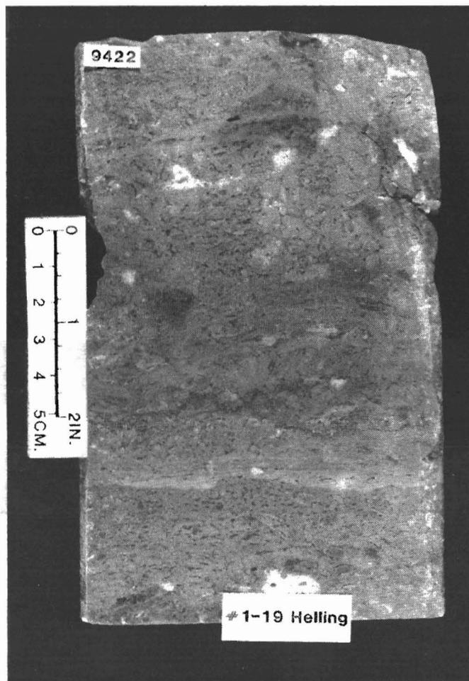
Figure 10a. (Facies 4). A peloidal and coated grain packstone with occluded fenestral fabric is part of the shoal facies of the Flat Lake subinterval. The large white patches are anhydrite and baroque dolomite cements. Transco, #1-19 Helling, SESEsec 19, T150N, R101W.
