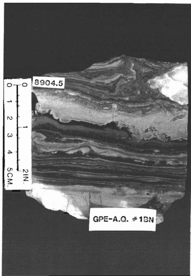
Figure 12a. (Facies 6). Wavy laminated dolomudstone of the intertidal-supratidal facies of the Flat Lake sub-interval. Some of the laminations may be stromatolites. Note the displacive anhydrite nodule at upper right indicating proximity to the sabkha. Sample from the GPE Al Aquitaine, #1 B.N., SESEsec 9, T146N, R103W.
