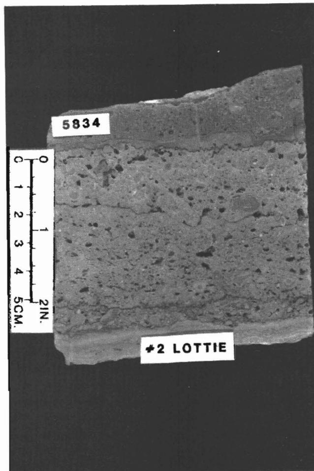
Figure 8. (C) 5834' Oolite-pisolite grainstone, Coteau interval. Some open fenestral pores, several stylolites, crust at base.
