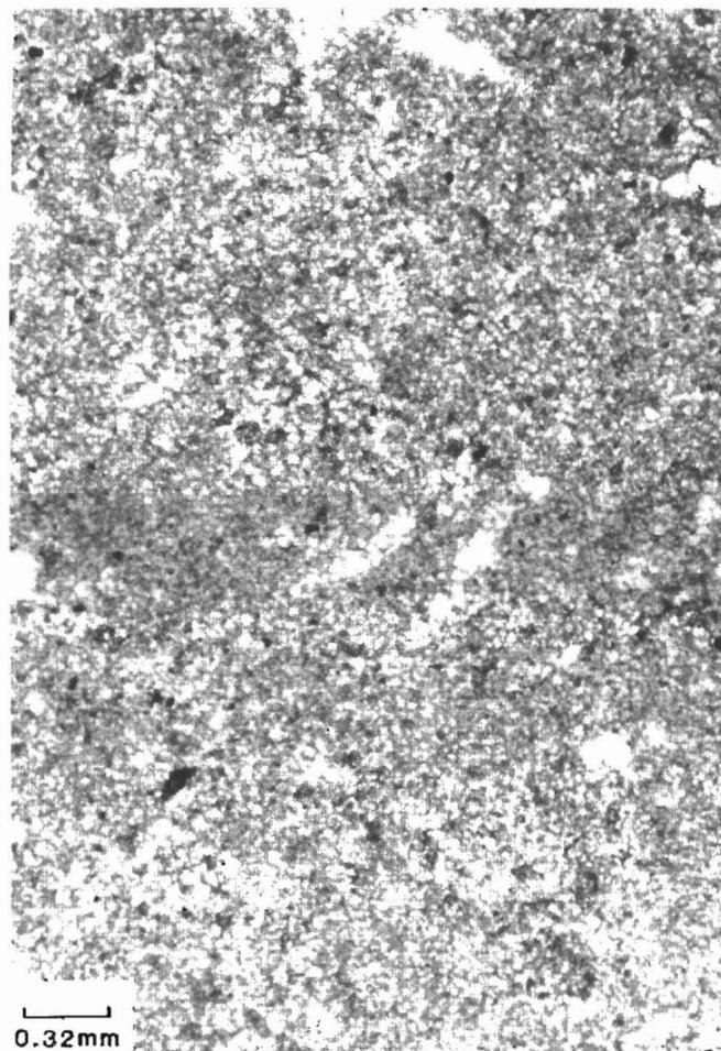
Figure 8b. (Facies 2). Dolomitization has produced sparse inter-crystalline porosity in this restricted subtidal sample. From 9178 feet in the Sun Exploration and Production, #2 Erickson, MNNEsec 27, T152N, R102W. The dark specks in this photomicrograph are small pyrite crystals.
