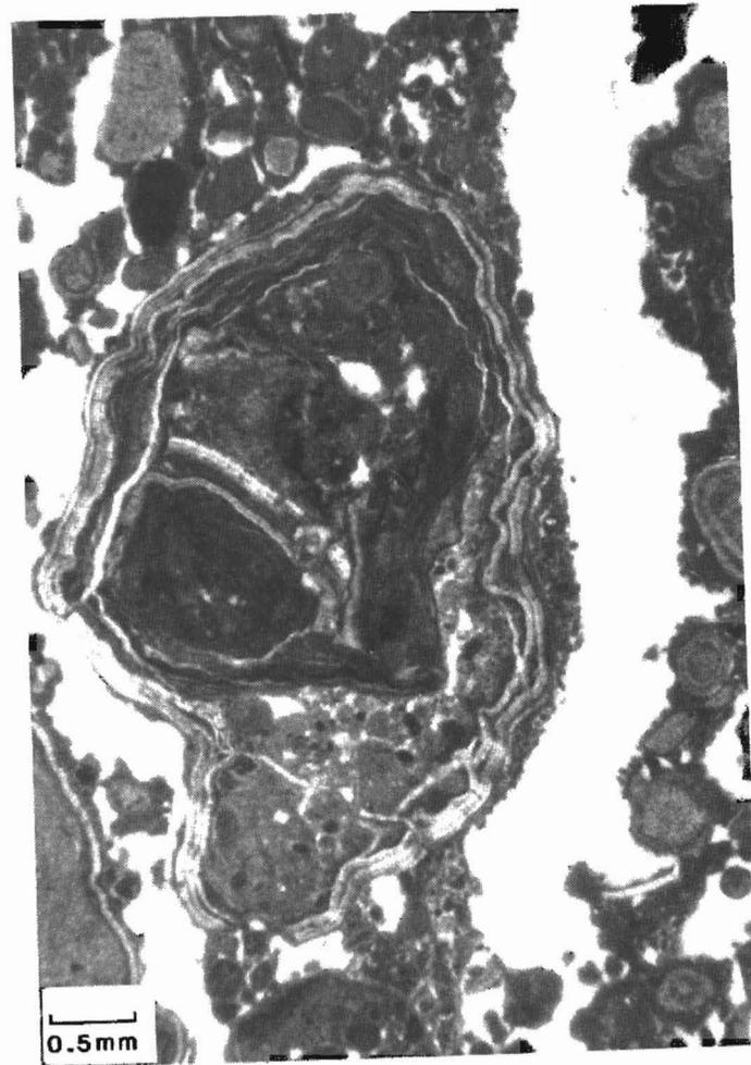
Figure 11d. (Facies 4). A large composite grain (center) shows multiple coatings indicating a complex origin. The occluded fenestral pore at right contains both fibrous calcite, lining the exterior of the pore, and sparry calcite which lines the interior. Sample from 9396 feet in the Superior, #1 Monson, NWSWsec 35, T152N, R102W.
