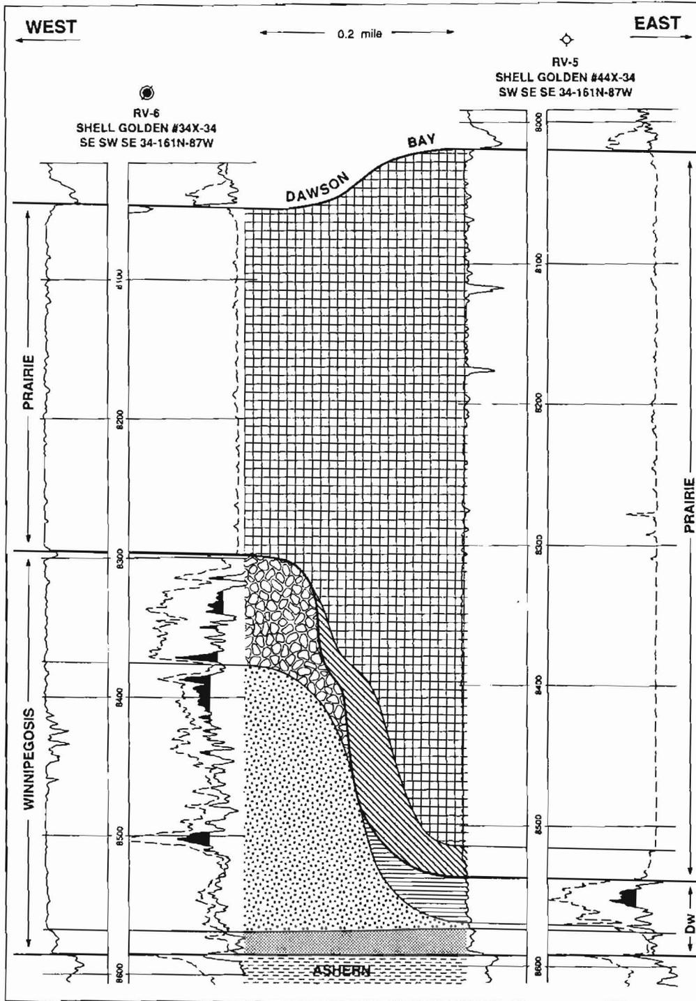
Fig. 13 - Stratigraphic and facies cross section of the Golden pinnacle reef, Renville County. Refer to Fig. 13 for summary of reef facies. Off-reef facies include basin laminite (horizontal ruled), Prairie anhydrite (diagonal ruled) and Prairie halite. Darkened portions of logs indicate  $\geq 8\%$   $\emptyset$ .
