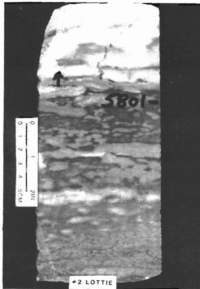
Figure 6. (B) 5801' Probisher Anhydrite. Note similarity of form to mottled dolomite at 5824'.
