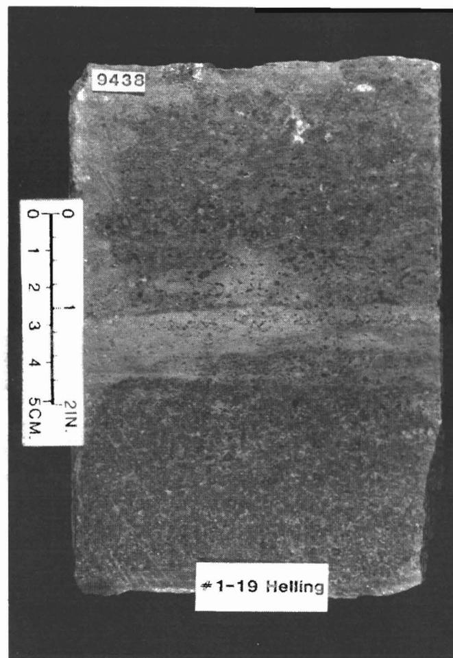
Figure 10b. (Facies 4). A peloidal and coated grain grainstone at the base of the sample grades upward into a wackestone. The grainstone bed is capped by a thin lime mudstone laminae which was probably produced by fall-out sedimentation during slack water deposition, from the Transco, #1-19 Helling, SESEsec 19, T150N, R101W.
