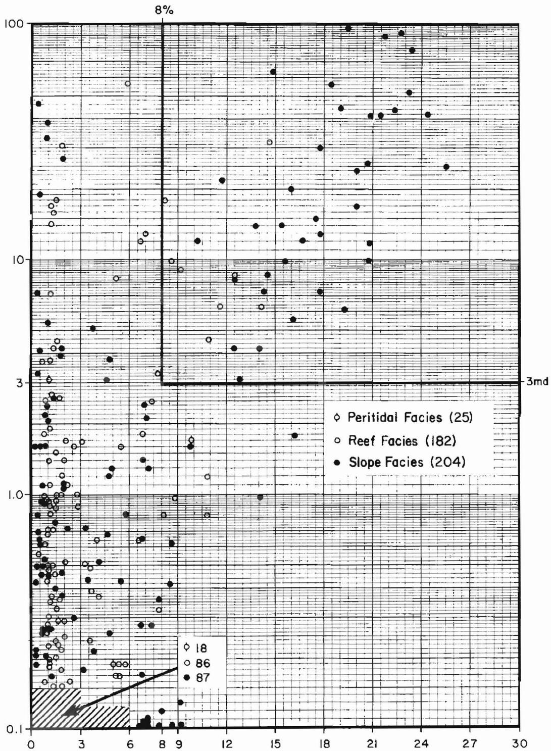
Fig. 11 -  $\phi$ -k plots for 411 core analyses from six wells on the Western Platform margin. 8% porosity and 3 md permeability denote approximate lower reservoir limits.
