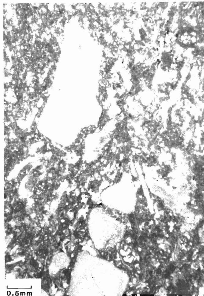
Figure 6b. (Facies 1). A photomicrograph of skeletal fragments typical of the shallow shelf facies. From 8767 feet in the Arco, #1 State Gafkjen, SESEsec 36, T158N, R100W.
