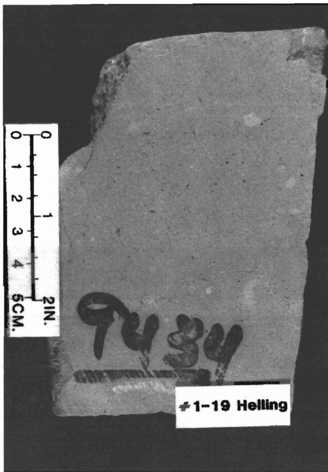
Figure 9a. (Facies 3). Massive-appearing lime mudstone from the restricted subtidal facies of the Flat Lake subinterval in the Transco #1-19 Helling, SESEsec 19, T150N, R101W. Massive appearance may be due to complete bioturbation. Porosity in this facies is locally good, but permeability is normally poor due to poor interconnection of pores.
