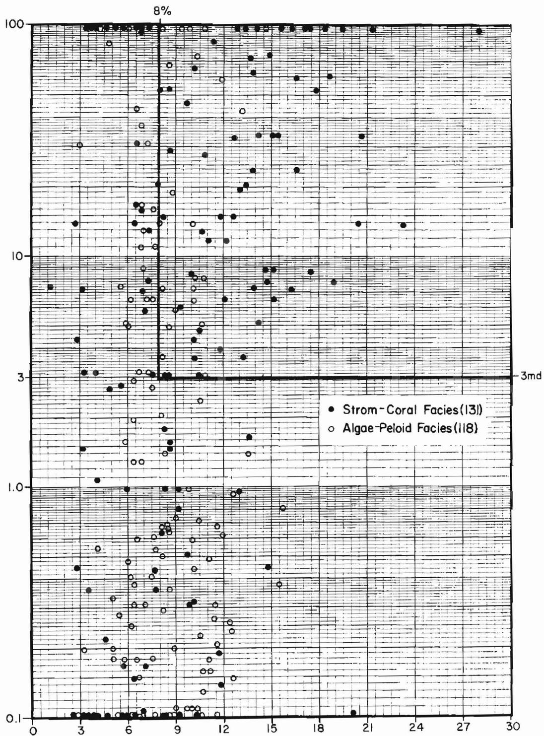
**Fig. 18** -  $\phi$ -k plots for 249 core analyses from three wells penetrating pinnacle reef facies. 8% porosity and 3 md permeability denote approximate lower reservoir limits.
