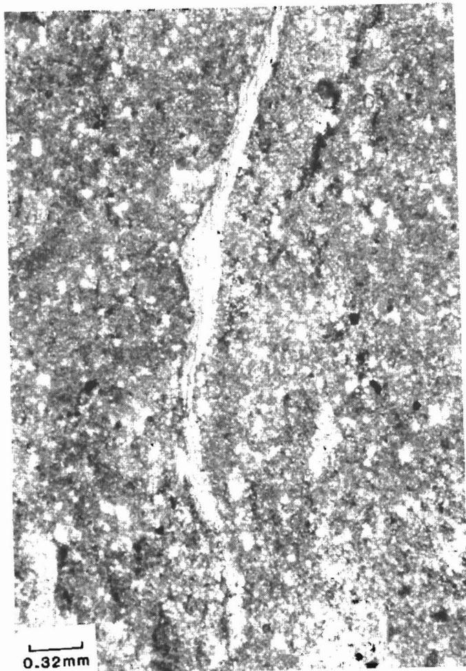
Figure 8c. (Facies 2). An elongate brachiopod fragment is well preserved in this slightly dolomitic mudstone. Dolomite has selectively replaced the lime mud fraction of this sample from 8738 feet in the Arco, #1 State Gafkjen, S8SEsec 36, T158N, R100W.
