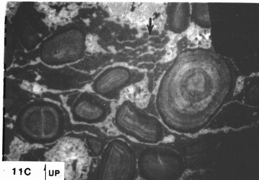
Figure 11. (C) Desiccation cracks subsequently infilled with drusy and blocky calcite cement, 2 Lottie well, 5946 ft. Photographs courtesy of Sue T. Reid.
