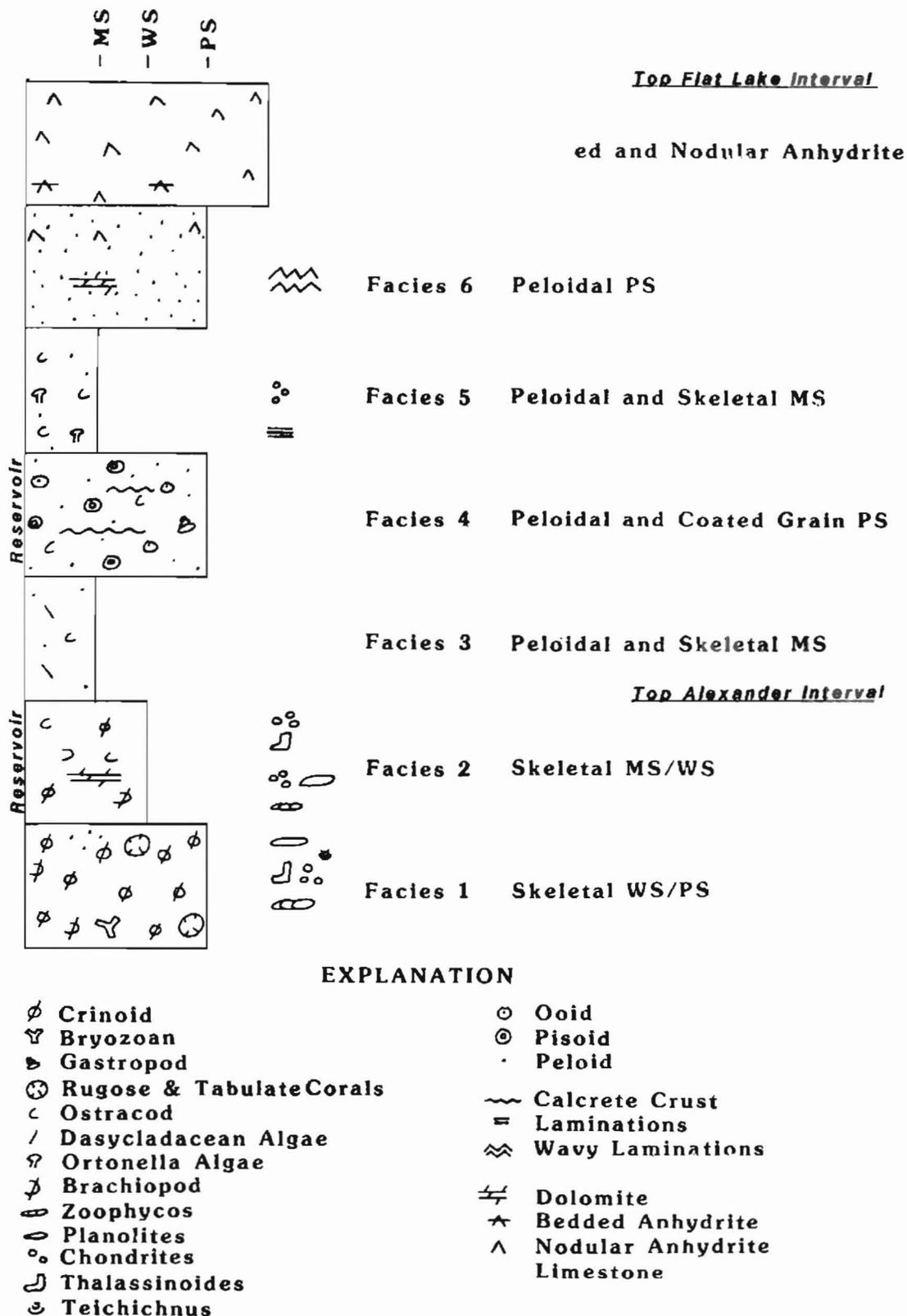
Figure 4. Type stratigraphic section from the Alexander and Flat Lake intervals in the central basin. Production in the Alexander interval is from dolomitic wackestones, while Flat Lake production is from lime packstones. Facies shown correspond to those discussed in the text.
