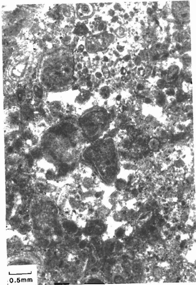
Figure 11c. (Facies 4). Intergranular pores are occluded with fibrous calcite cement in this packstone from 8045 feet in the Depco, #44-16 Larson, SESEsec 16, T159N, R102W. Baroque dolomite cement (large white spots) has further reduced porosity and permeability in this sample.
