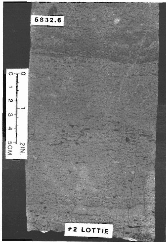
Figure 8. (A) 5832' Fenestral porosity almost completely infilled with blocky calcite cement, Coteau interval.
