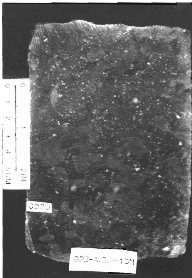
Figure 6a. (Facies 1). A burrowed and skeletal wackestone. Burrow structures are of the *Cruziana* ichnofacies, which are part of the shallow shelf, GPE, #1 BN, SESEsec 1, T147N, R105W.
