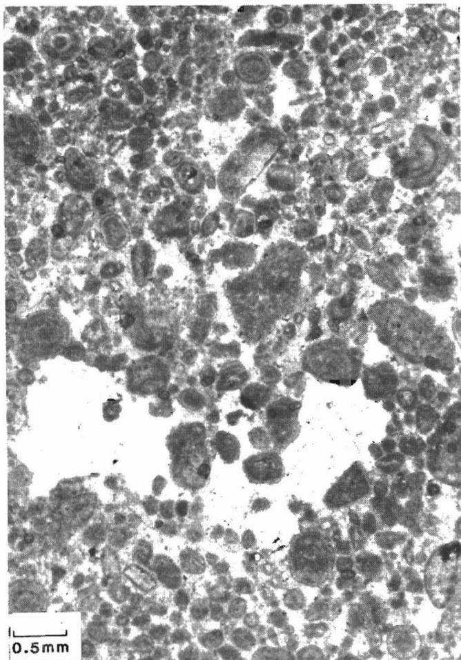
Figure 11a. (Facies 4). Fibrous calcite occludes intergranular porosity in this peloidal and ooiditic packstone. The large vuggy pore at the base of this photomicrograph is occluded with prismatic calcite spar and baroque dolomite cements. Sample is from 8045 feet in the Depco, #44-16 Larson, SESEsec 16, T159N, R102W.
