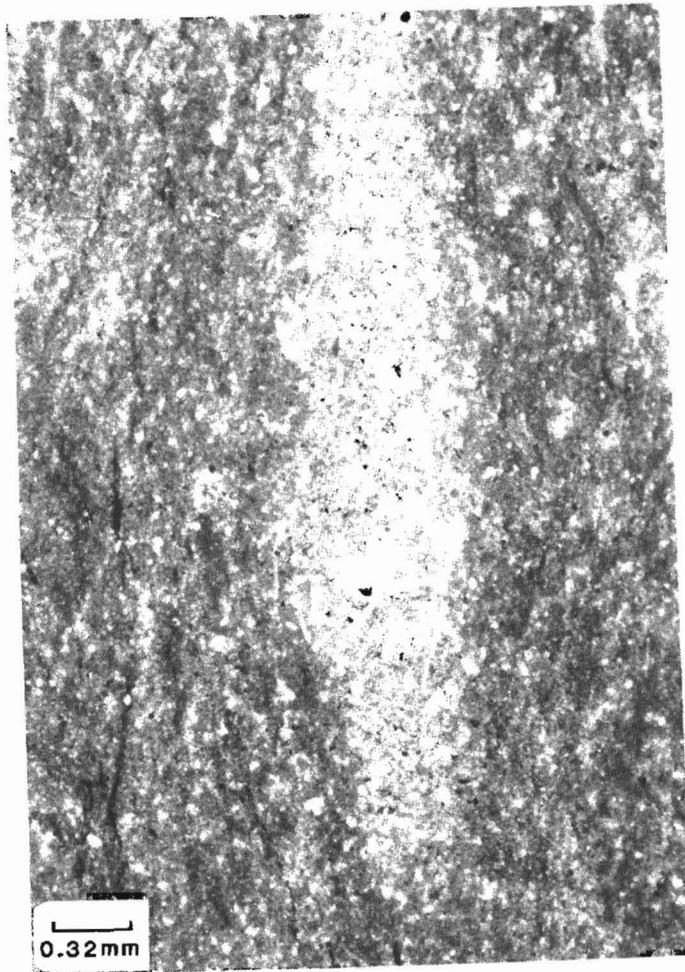
Figure 8d. (Facies 2). The lime mudstone within a *Chondrites* burrow structure has been preferentially replaced by dolomite in this photomicrograph from 9441 feet in the Superior, #1 Monson, N8Wsec 35, T152N, R102W. This is the principal reservoir type in the Alexander sub-interval.
