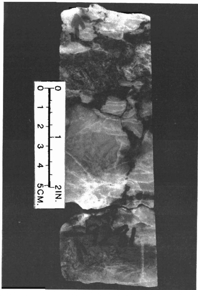
Figure 13a. (Facies 7). Nodular anhydrite from a sabkha sequence in the Depco-Pennzoil, #22-32 Federal, SWNEsec 22, T147N, R101W.
