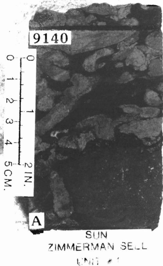
Figure 7c. (Facies 2). Large Thalassinoides burrow structures in a slightly dolomitic mudstone, from the Sun Exploration and Production, #1 Zimmerman Seel, SWNEsec 3, T152N, R104W.
