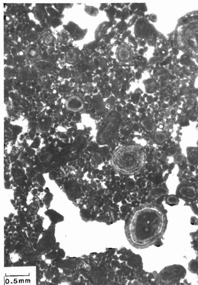
Figure 10d. (Facies 4). A photomicrograph from a shoal sequence shows small peloids and various sizes of coated grains. Fenestral pores are occluded with prismatic calcite spar and baroque dolomite cements. Sample from 9144 feet in the Sun Exploration and Production, #2 Erickson, NWNWsec 27, T152N, R102W.
