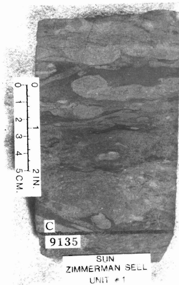
Figure 7d. (Facies 2). Thalassinoides and Teichichnus burrow structures in the restricted subtidal, Sun Exploration and Production, #1 Zimmerman Seel, SWNEsec 3, T152N, R104W.
