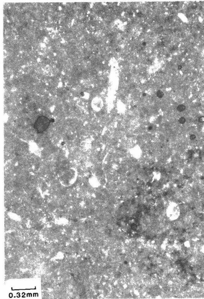
Figure 9d. (Facies 3). Another example of restricted subtidal deposition from the Flat Lake subinterval shows very small skeletal fragments (mostly ostracods and calcispheres) in a lime mudstone matrix. Some of the small white specks are dolomite rhombohedrons. Sample from 9185 feet in the Sun Exploration and Production, #1 D. Erickson, SE<sub>4</sub>NW<sub>4</sub>sec 27, T152N, R103W.
