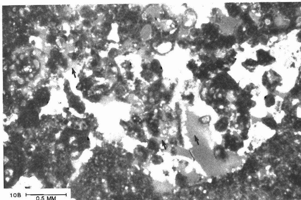
Figure 10. (A) Oolith-pisolith grainstone, 1 Marvin well, SE8Wsec 12, T163N, R91W, 5777.5 ft. Note drusy calcite lining fenestral pores which are partially to completely infilled with blocky calcite (labelled "C" on photo). (B) Bioclastic packstone and grainstone, 2 Galvin well, NWNWsec 12, T163N, R91W, 5318.5 ft. Note good interparticle porosity.
