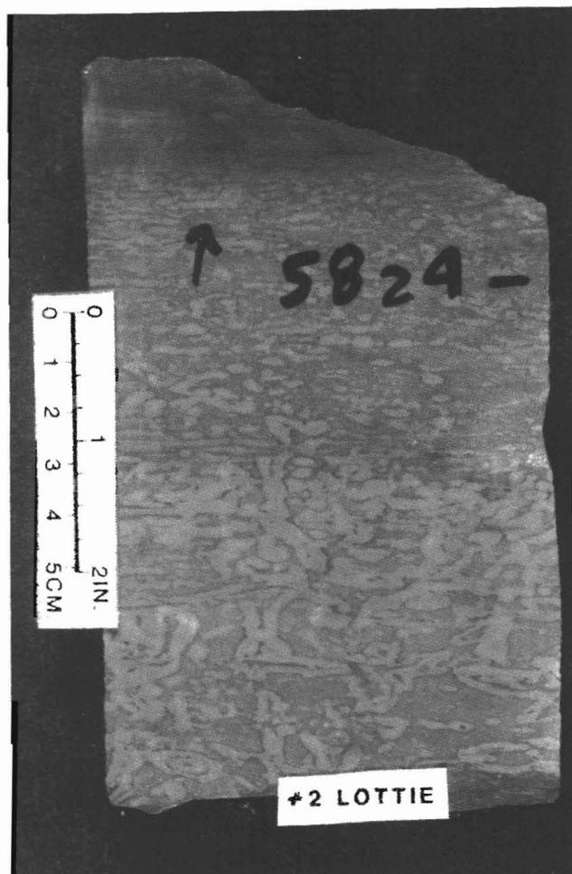
Figure 7. 5824'. Mottled (pattern) dolomite in State A marker
