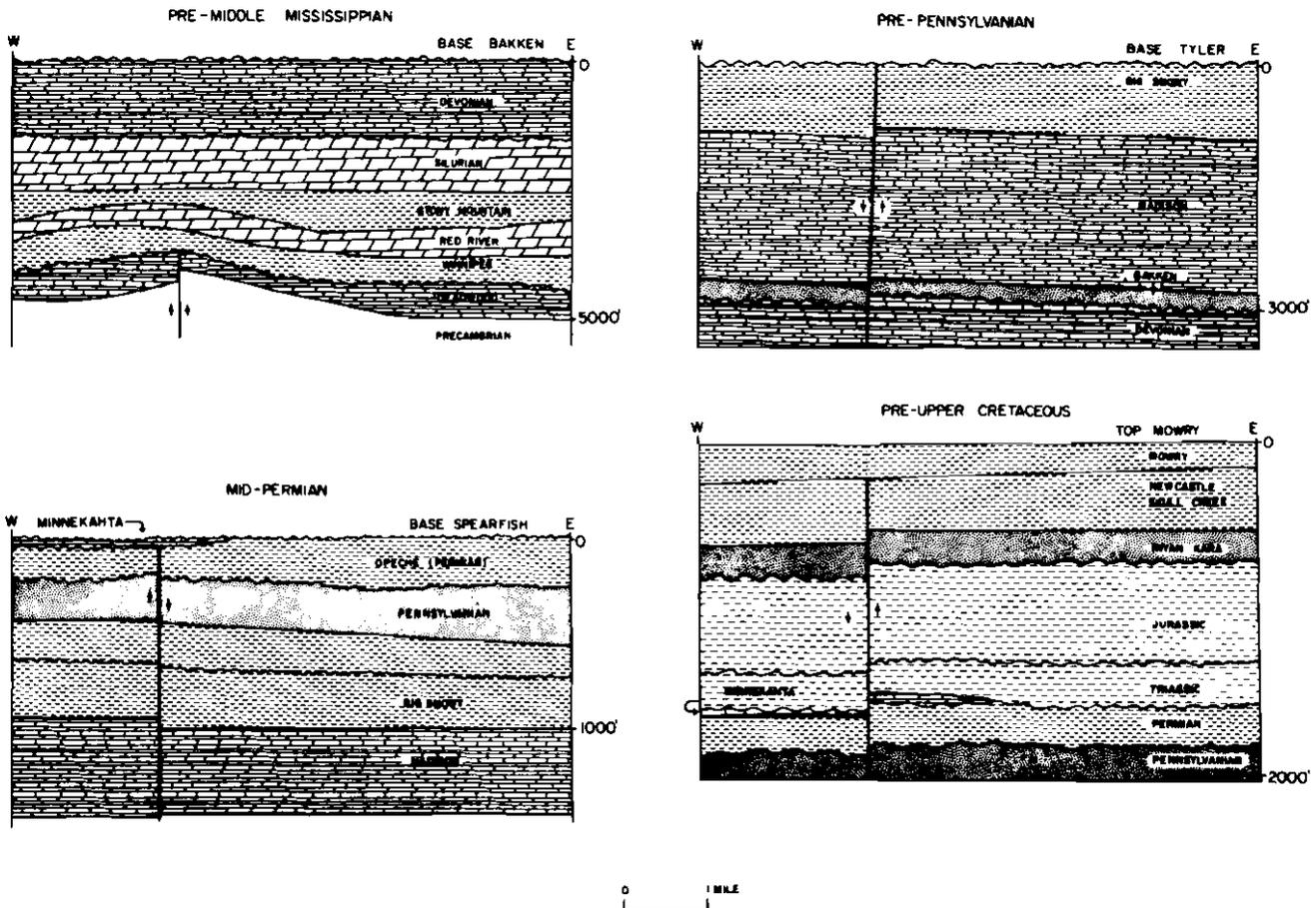
FIG. 17—Diagrammatic cross sections of Nesson anticline showing structural development. Note apparent reversal of fault movement during mid-Permian. Some of pre-Upper Cretaceous movement may be related to salt solution.
