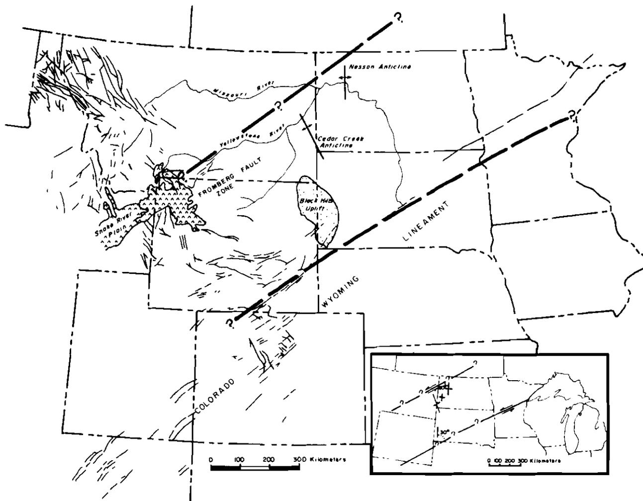
FIG. 24—Diagram showing relationship of Fromberg-Colorado-Wyoming shear zones to structural features of Rocky Mountains and Williston basin.
