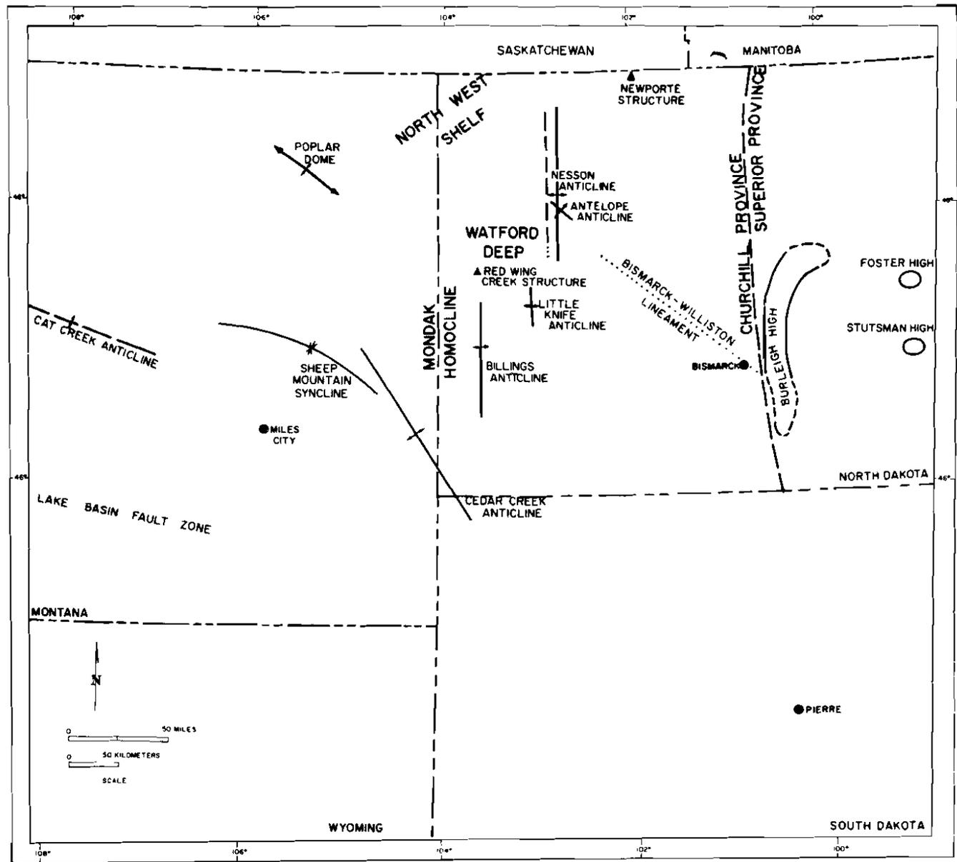
FIG. 2—Major structures of Williston basin based on current subsurface structural mapping and geophysical interpretations.
