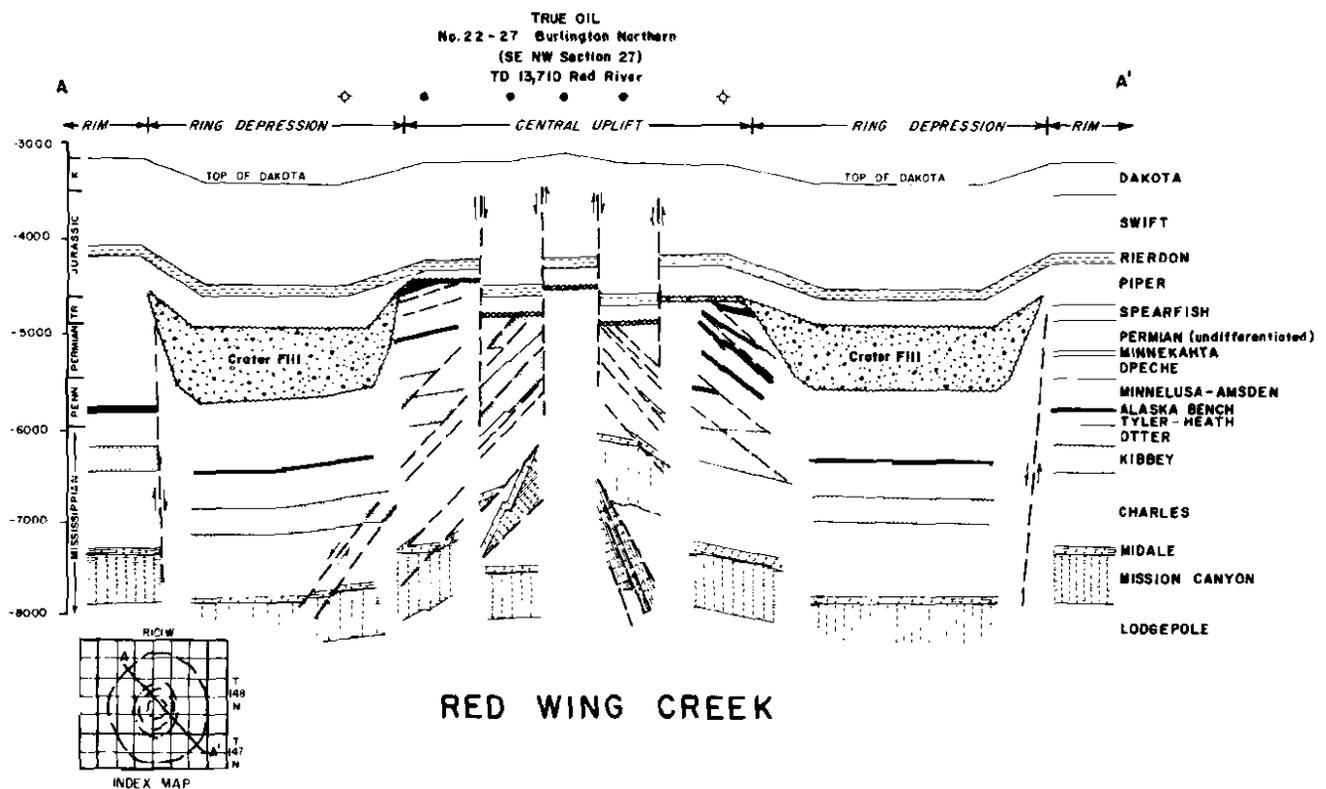
FIG. 21—Cross section through Red Wing Creek structure, McKenzie County, North Dakota, demonstrating meteorite-impact hypothesis for origin of this structure. True Oil 22-27 Burlington Northern discovery well was drilled on top of central uplift. Modified from Exhibit 6, case 1152, North Dakota Industrial Commission, submitted by Union Oil Co. of California.
