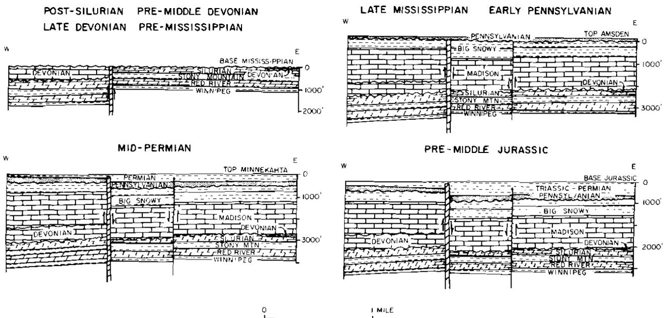
**FIG. 20**—Diagrammatic cross sections across Cedar Creek anticline at Gas City field. Modified from Clement (1976). Minor second fault generated locally in Gas City area during Late Mississippian-Early Pennsylvanian episode was concurrent with minor reversal of movement on principal west fault zone.
