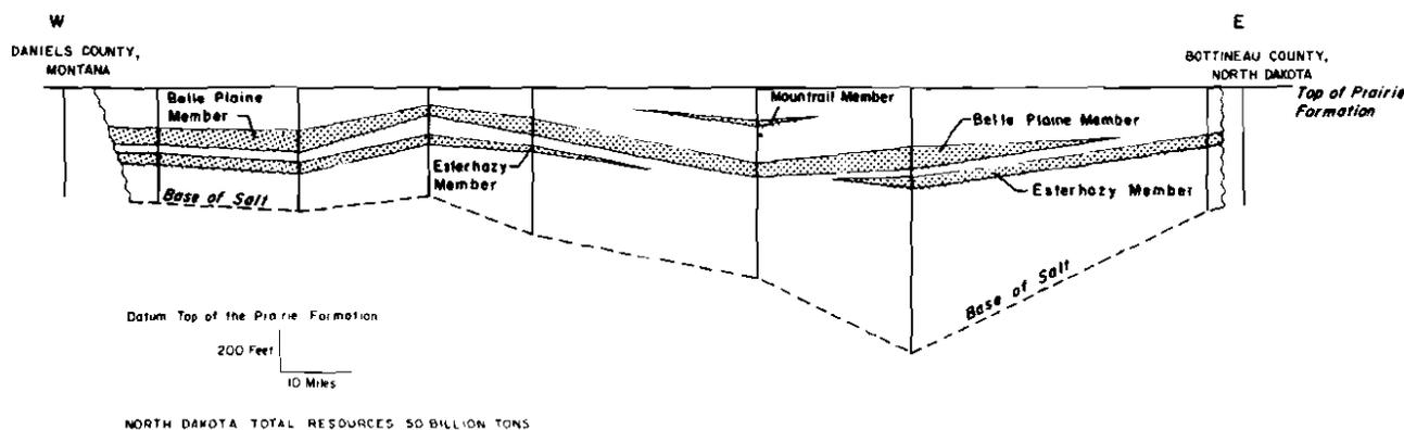
FIG. 32—Cross section from Daniels County, Montana, through Bottineau County, North Dakota, showing potash beds within Prairie Formation. Shaded zones are potash bearing. Modified from Anderson and Swinehart (1979).
