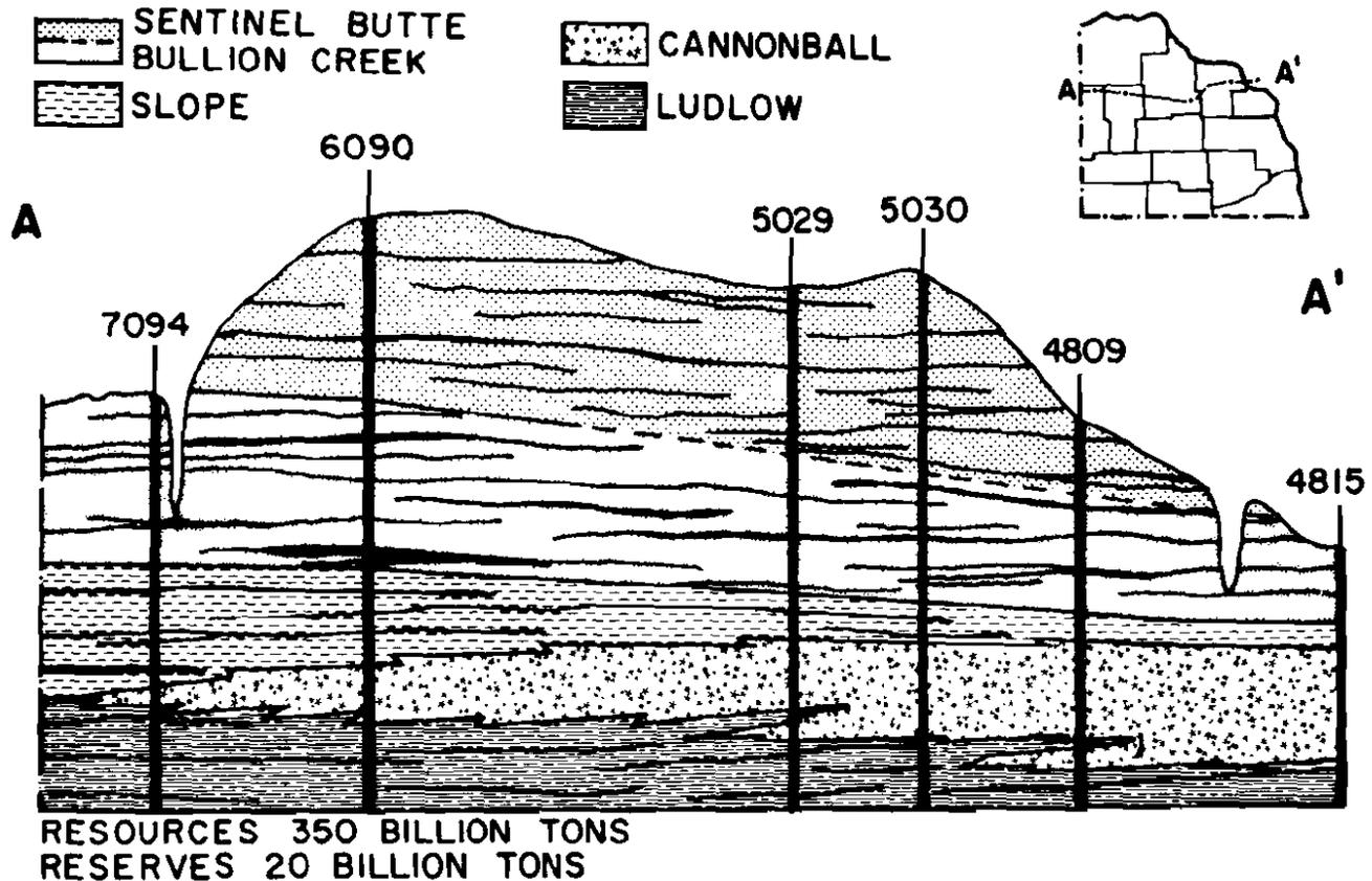
FIG. 34—Diagrammatic cross section of Paleocene rocks in western North Dakota showing relationship of lignite beds and stratigraphic units. Numbers at vertical dark lines refer to North Dakota Geological Survey drill-hole control.
