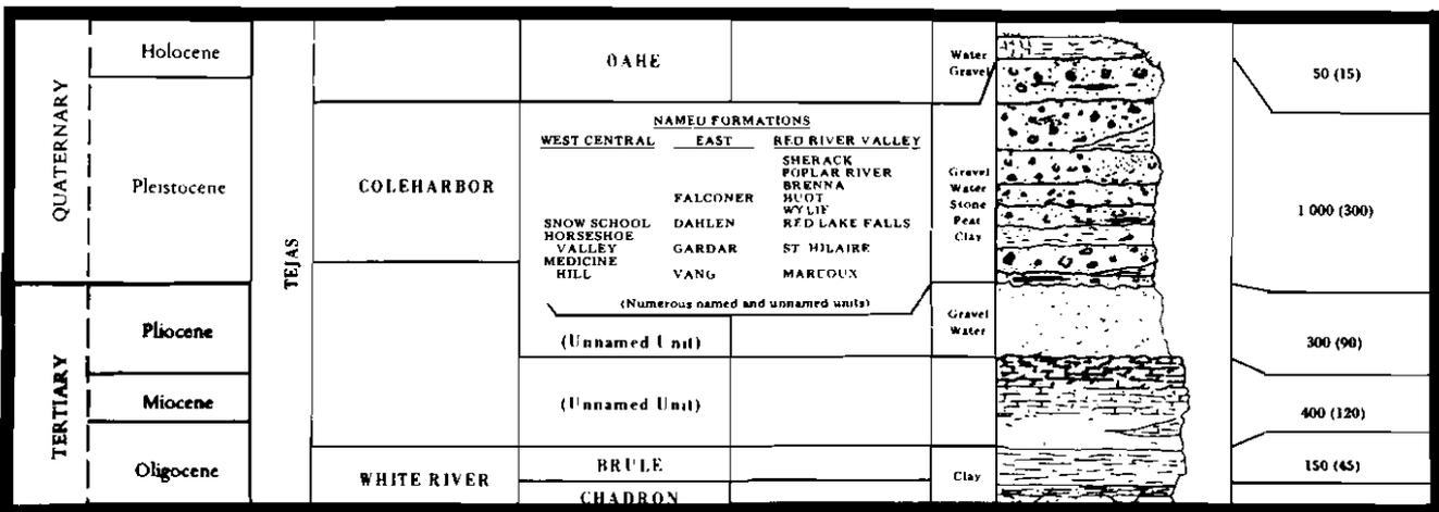
FIG. 15—Stratigraphic section of Tejas sequence rocks and sediments.
