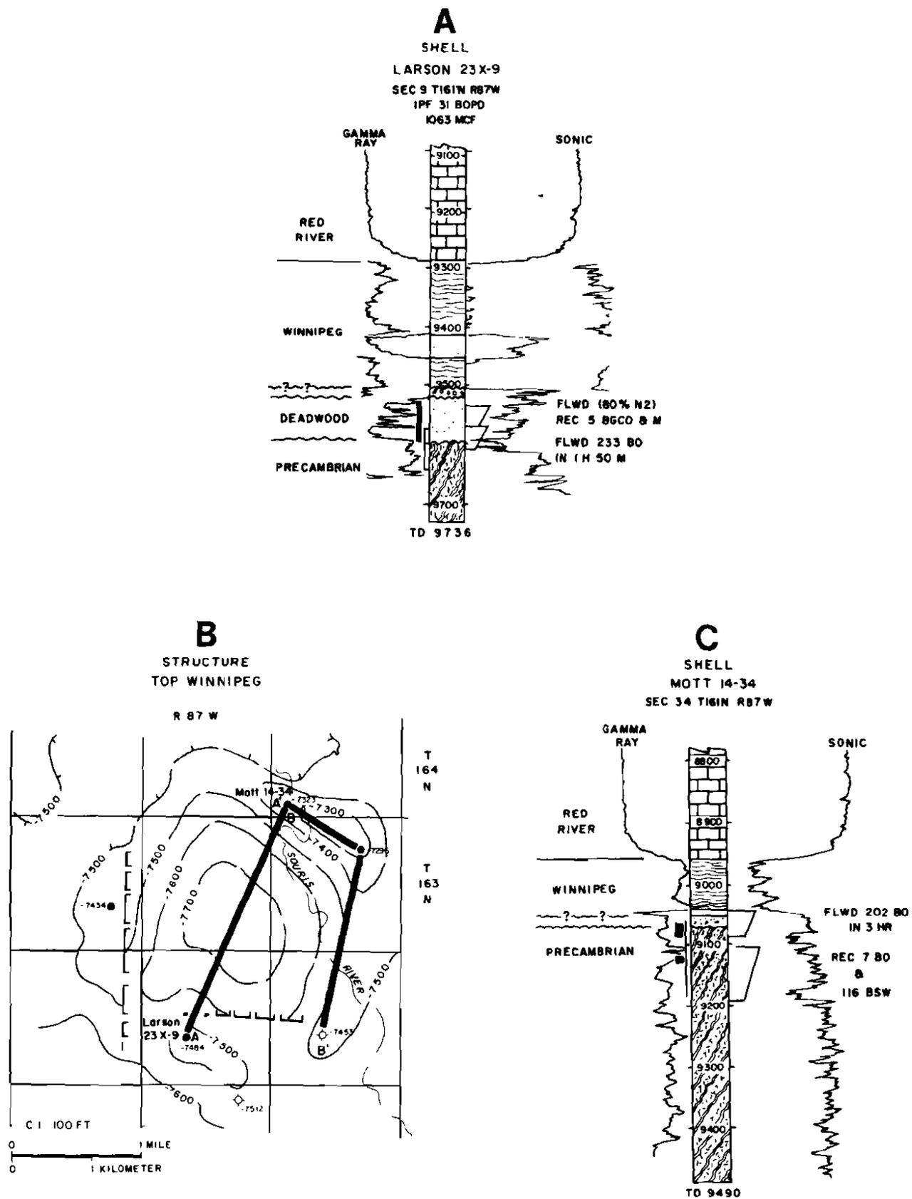
FIG. 22—Newporte field structure map and lithologic sections. A. Shell Larson 23 X-9, showing producing interval in Deadwood Formation. B. Structure of top of Winnipeg Formation in Newporte field. C. Shell Mott 14-34, showing producing intervals in Precambrian and at Winnipeg Precambrian contact. Modified from Clement and Mayhew (1979).
