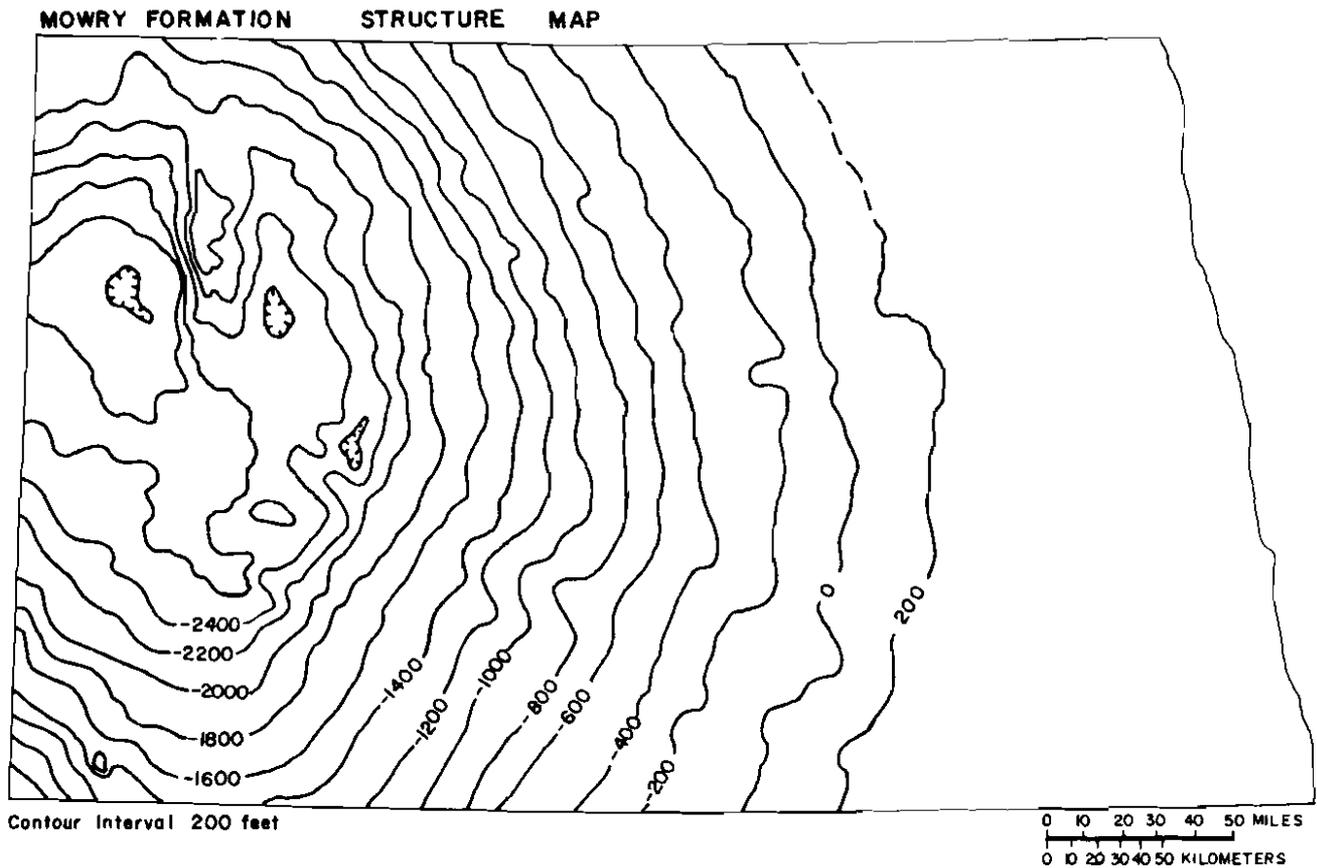
**FIG. 19**—Structure map of top of Mowry Formation (Cretaceous). Compare Figure 18. Closely spaced contours on west side of Nesson anticline suggest post-Mowry faulting on that structure. Bismarck-Williston trend also appears to be well developed as is Billings anticline. Little Knife anticline does not appear to be so well defined at this horizon.
