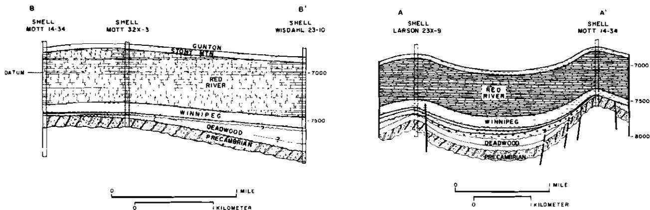
FIG. 23—Cross sections across Newport field. See Figure 22 for lines of section. Modified from Clement and Mayhew (1979).
