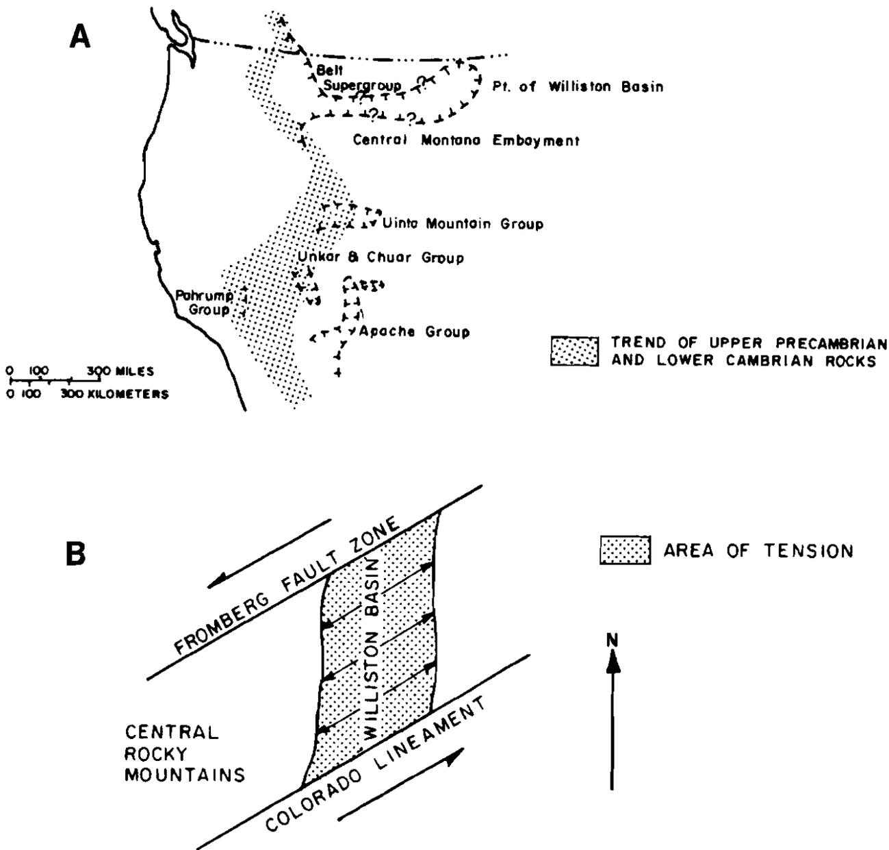
FIG. 25—A. Aulacogen origin for Williston basin. Basin is shown as possible extension of Central Montana embayment during Precambrian time. Modified from Stewart (1972). B. Pull-apart origin for Williston basin. Basin was placed under tension due to movement along major shear zones causing grabenlike downdropped blocks. Modified from Burchfiel and Stewart (1966).
