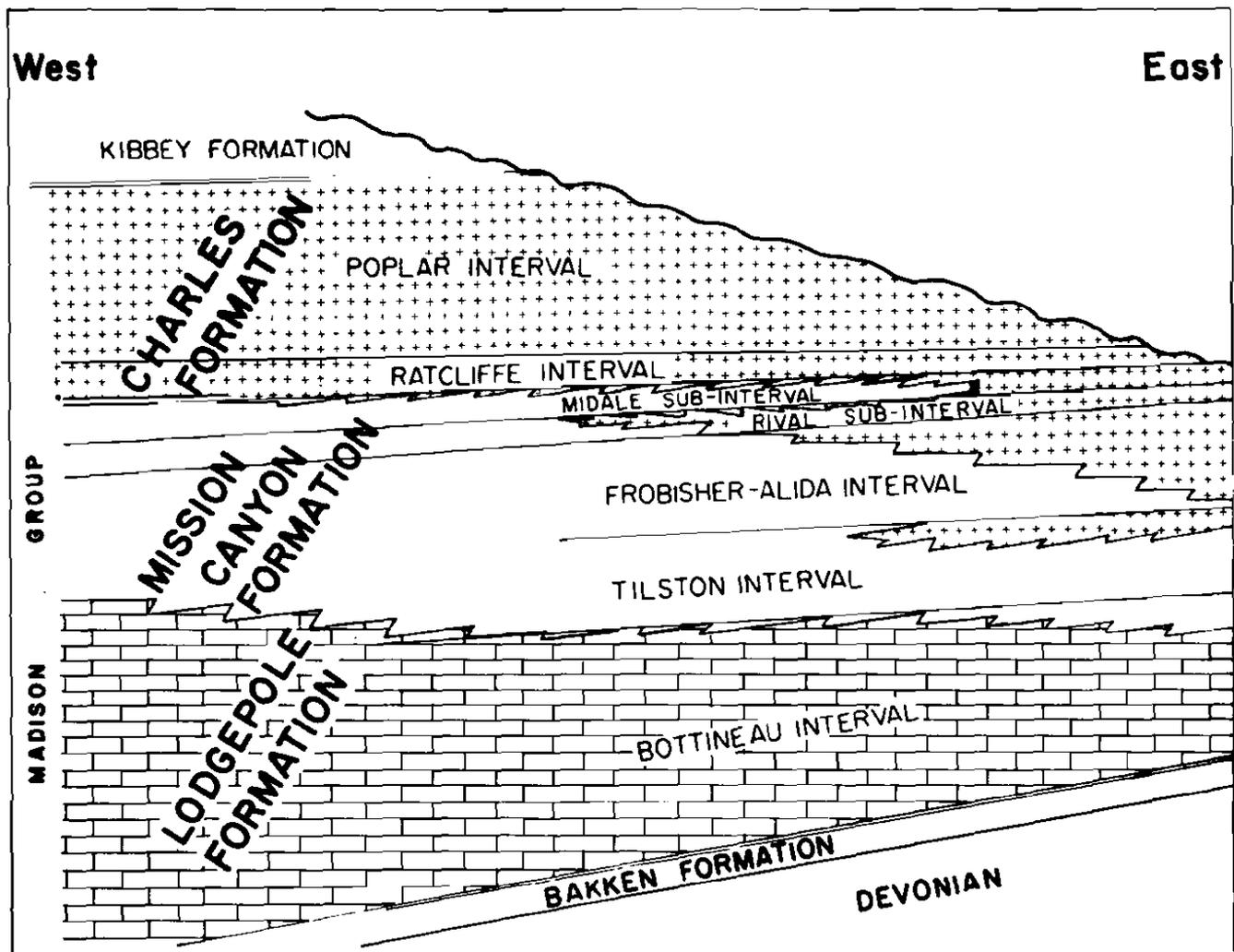
FIG. 11—Generalized cross section of Mississippian rocks in Williston basin showing relationship of facies and stratigraphic nomenclature. Modified from Carlson and Anderson (1966).
