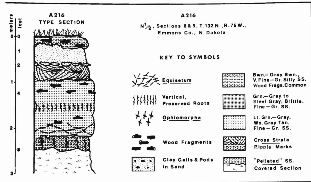
Figure 2. Schematic type section of Linton Member.
