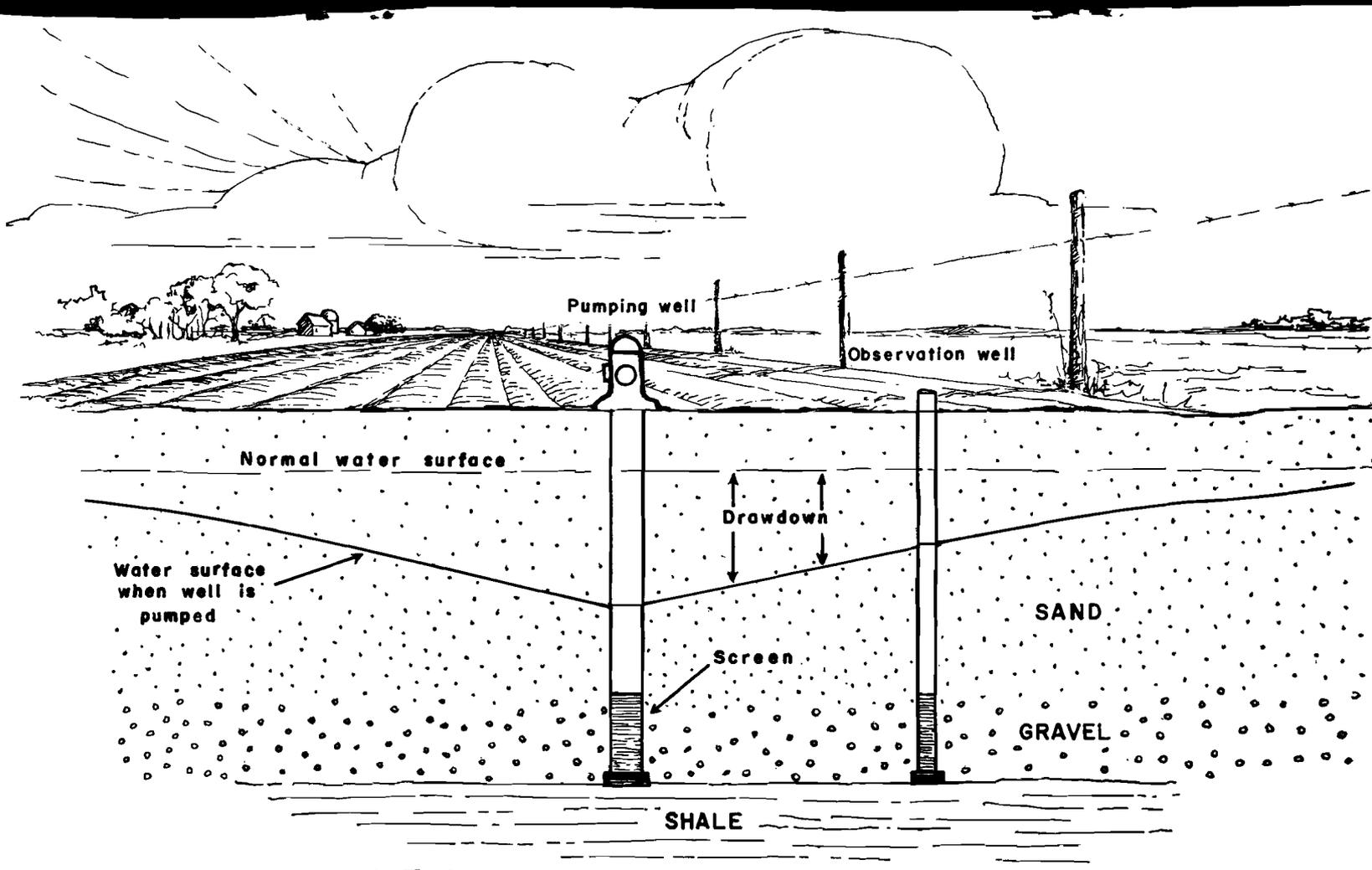
FIGURE 6. SUBSURFACE CONDITIONS IN VICINITY OF PUMPING WELL
