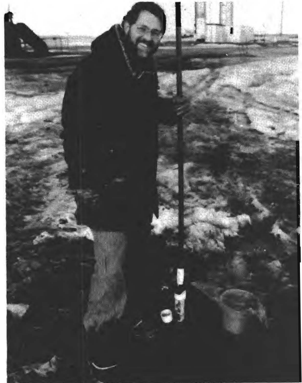
Figure 6. David O. Lechner obtaining groundwater samples from a Winderl piezometer.
