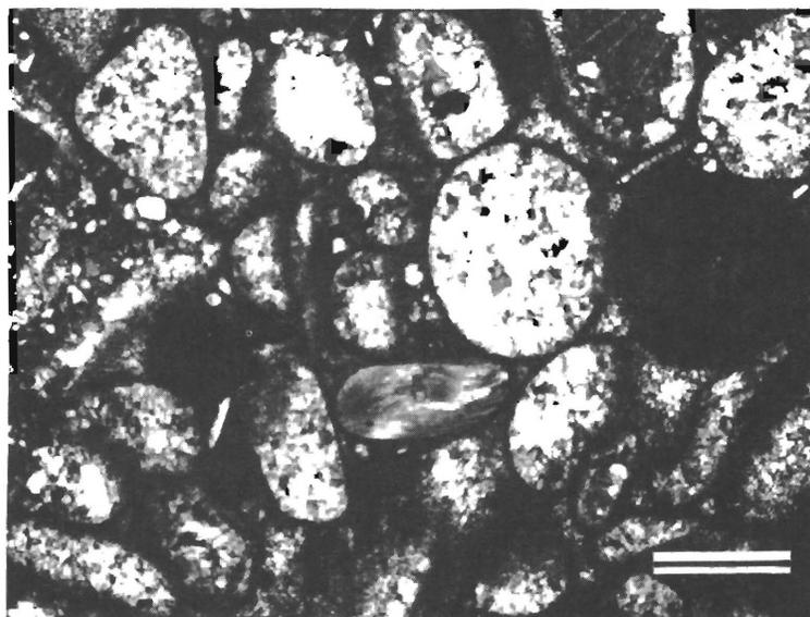
Figure 18. Photomicrograph of a thin section taken normal to the length of the core showing the discoid shape of the allochems. Thin-section number 5135.4, 25X. Bar represents .5 mm.
