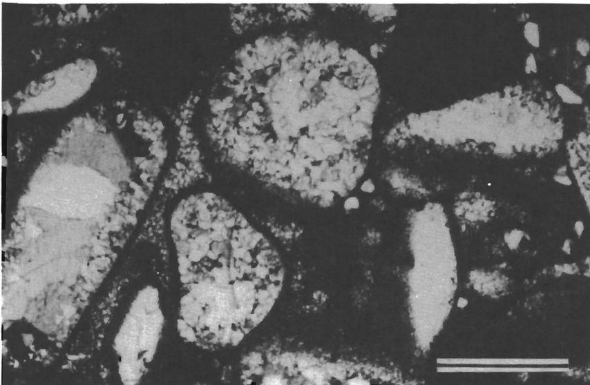
Figure 22. Photomicrograph of calcite cement infilling molds of mollusk grains. Thin-section number 5181.1, 40X. Bar represents .5 mm.
