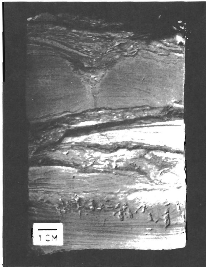
Figure 29. Core slab of a laminated and bioturbated mudstone. 5061.6 to 5061.2 feet.
