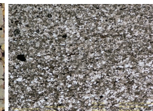
Interbedded siltstone and very fine-grained quartz sandstone sequence with calcite cement. Limited interparticle porosity due to dolomitization of the calcite cement.
