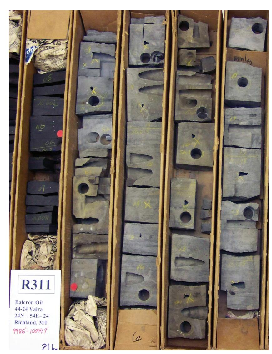
Balcron Oil - 44-24 Vaira (SESE Sec 24, T24N, R54E) – Depths 10,005.5 to 10019.5 ft. - Base of the Upper Member through the reservoir section (Log below; USGS Photograph).
