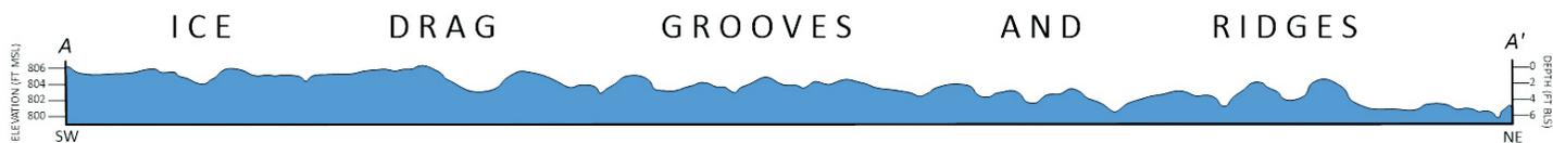
**FIGURE 8.** Topographic section A to A' from LiDAR surface model of the ice-drag features noted in Figure 5. Local relief on these grooves and ridges is only a few feet. This profile has been considerably stretched or exaggerated in the vertical scale to visualize these micro-relief features as the horizontal distance depicted here is over a mile.
