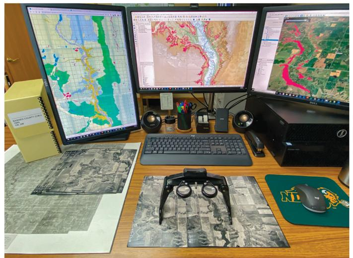
**FIGURE 2.** Phase II landslide mapping along the Sheyenne River Valley using 1:20,000-scale 1959 aerial photographs viewed through a stereoscope (bottom), a Barnes County surface geology map (left screen), LiDAR DEM (center screen), and aerial imagery on Google Earth (right screen).
