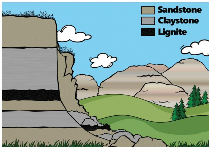
**FIGURE 10.** Graphic illustrating the generalized North Dakota badlands lithologies within a rotational landslide.
