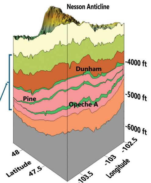
**FIGURE 1.** Stratigraphic column of the intervals containing the major shallow salts of the Williston Basin in North Dakota (Murphy et al., 2009). Salts are represented by the green cross hatch pattern in the rock column on the left and in green in the 3-D block diagram of the central basin on the right.
