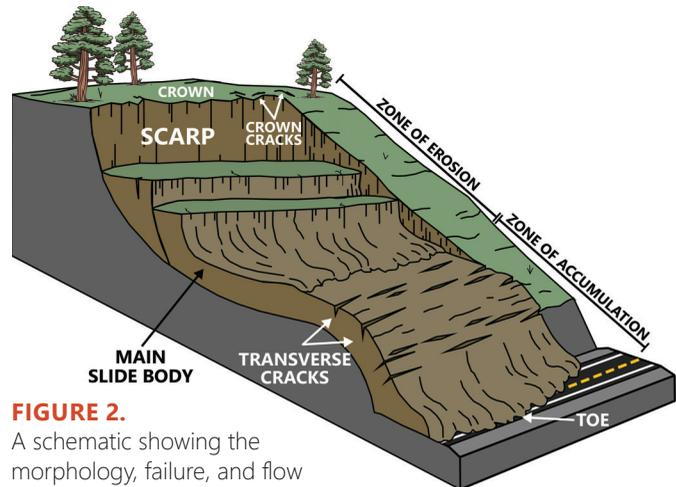
**FIGURE 2.** A schematic showing the morphology, failure, and flow mechanics of a rotational landslide. Modified from Bowman and Lund (2020) and Highland (2004).
