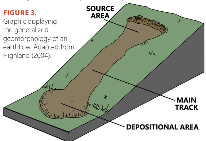
**FIGURE 3.** Graphic displaying the generalized geomorphology of an earthflow. Adapted from Highland (2004).
