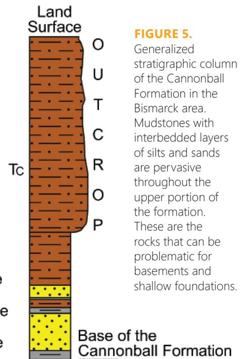
**FIGURE 5.** Generalized stratigraphic column of the Cannonball Formation in the Bismarck area. Mudstones with interbedded layers of silts and sands are pervasive throughout the upper portion of the formation. These are the rocks that can be problematic for basements and shallow foundations.
