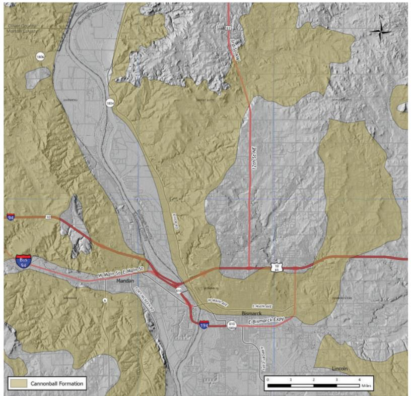
**FIGURE 4.** The Cannonball Formation (shaded in tan) is exposed at the land surface or buried just beneath a shallow layer of glacial sediments throughout the northern Bismarck-Mandan area. Future geologic investigations to better characterize this unit are planned.
