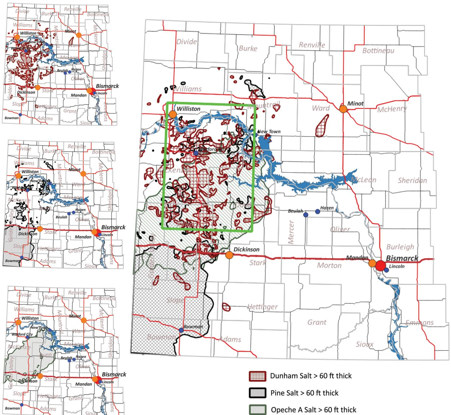
**FIGURE 2.** Maps of the individual shallow salts greater than 60 feet (left) and a map of the combined Dunham, Pine, and Opeche A salts with thicknesses greater than 60 feet (right). The green rectangle in the image on the right outlines the footprint of the 3D block diagram in figure 1.
