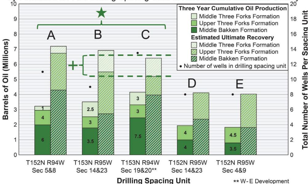
**FIGURE 3.** A comparison of the sum of the first three years' production and estimated ultimate recovery forecasts for the wells within five different drilling spacing units (A-E, locations on figure 4) in northeastern McKenzie County.
