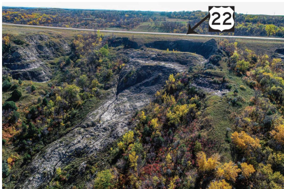
**FIGURE 11.** UAS photo displaying a landslide in the badlands of North Dakota. Note: the proximity of the landslide to Highway 22 (approximately 100 feet from the highway shoulder to the headscarp). UAS photo collected on October 8, 2019, by NDGS geologists Christopher Maiké and Levi Moxness.
