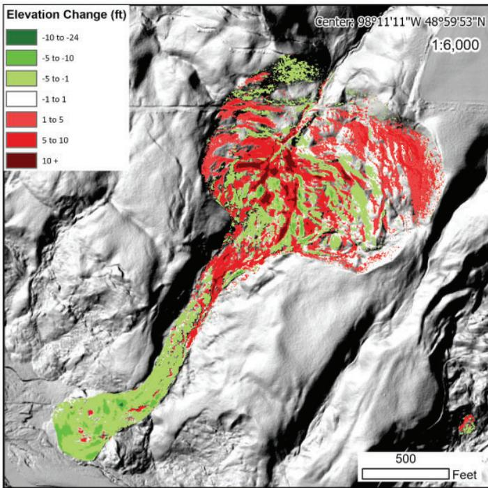
**FIGURE 8.** Earthflow located in the Pembina Gorge in northeast North Dakota. Overlain on the LiDAR base is the resulting LiDAR differencing raster. LiDAR was collected here in 2008 and 2018, meaning anything in red is a net loss in the z-direction (erosion) and anything in green is a net gain in the z-direction (deposition).
