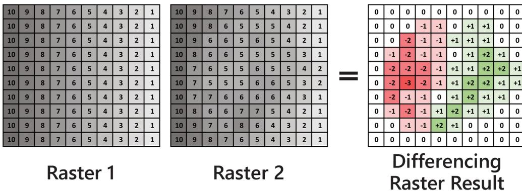
**FIGURE 7.** Diagram showing raster 2 being subtracted from raster 1. This would be an example of the “z-value” and observing any change, as seen in the “Differencing Raster Result.” This loosely portrays a landslide failure, with the red (net loss) being the scarp and downslope erosive movement and the green (net gain) being the downslope deposition and toe.
