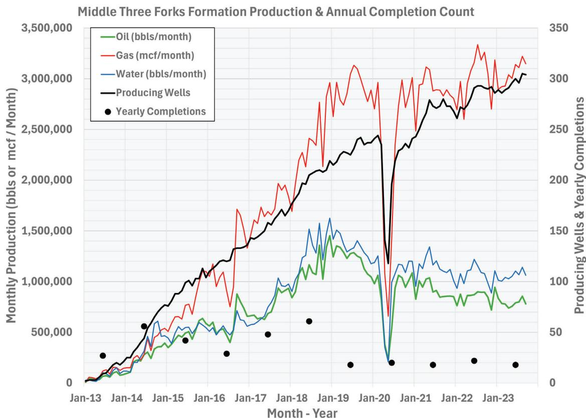
**FIGURE 1.** Monthly cumulative production of oil, gas, and water from middle Three Forks Formation horizontal wells, along with the active producing well count and the number of middle Three Forks Formation wells completed each year since the beginning of its development.
