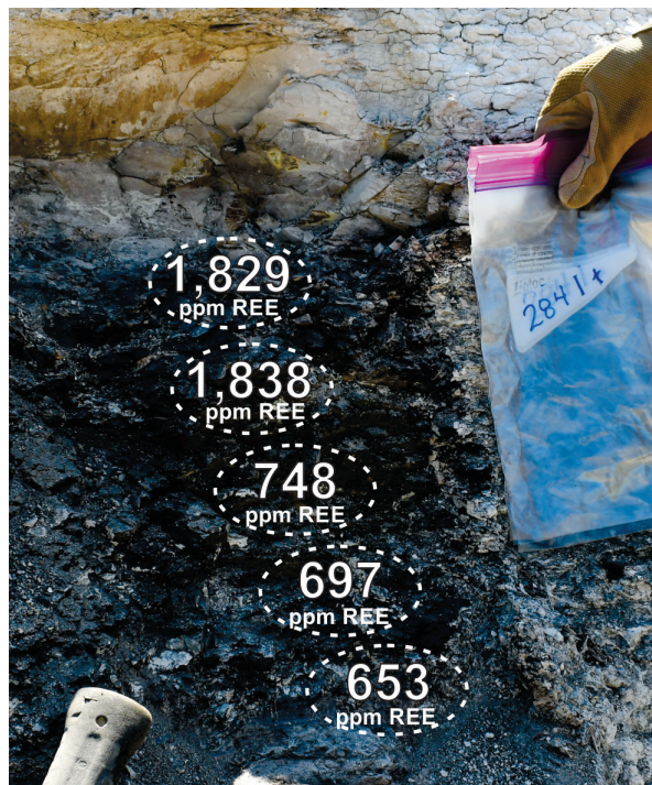
FIGURE 6. Sampling a 17-inch-thick lignite below the Rhame bed in southeastern Golden Valley County. Sample locations and total rare earth element (REE) concentrations plotted on the right.
