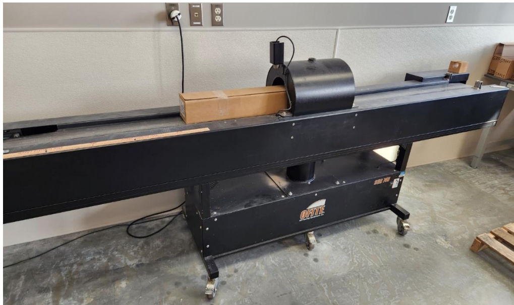
Pictured above: core gamma ray machine at the Wilson M. Laird Core & Sample Library. Upon request, a core library technician is available to run core samples through the core gamma ray machine and generate spectral core gamma ray curves.
