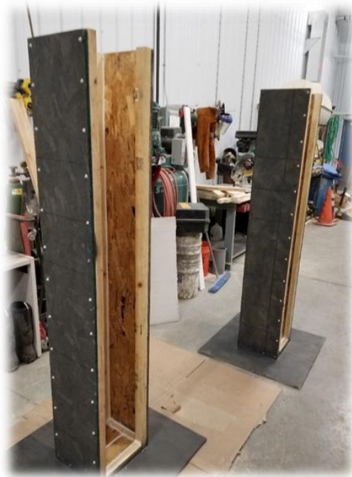
Images 10 & 11: Wood construction of the test columns.
