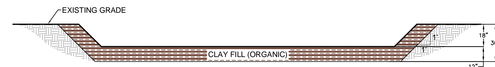
CONCEPTUAL TEST CELL PRC-1 - CROSS SECTION
