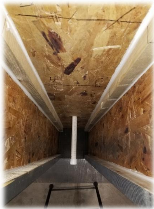
Images 10 & 11: Wood construction of the test columns.
