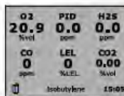
The MX6 clearly shows real-time readings in PPM or % by volume.
