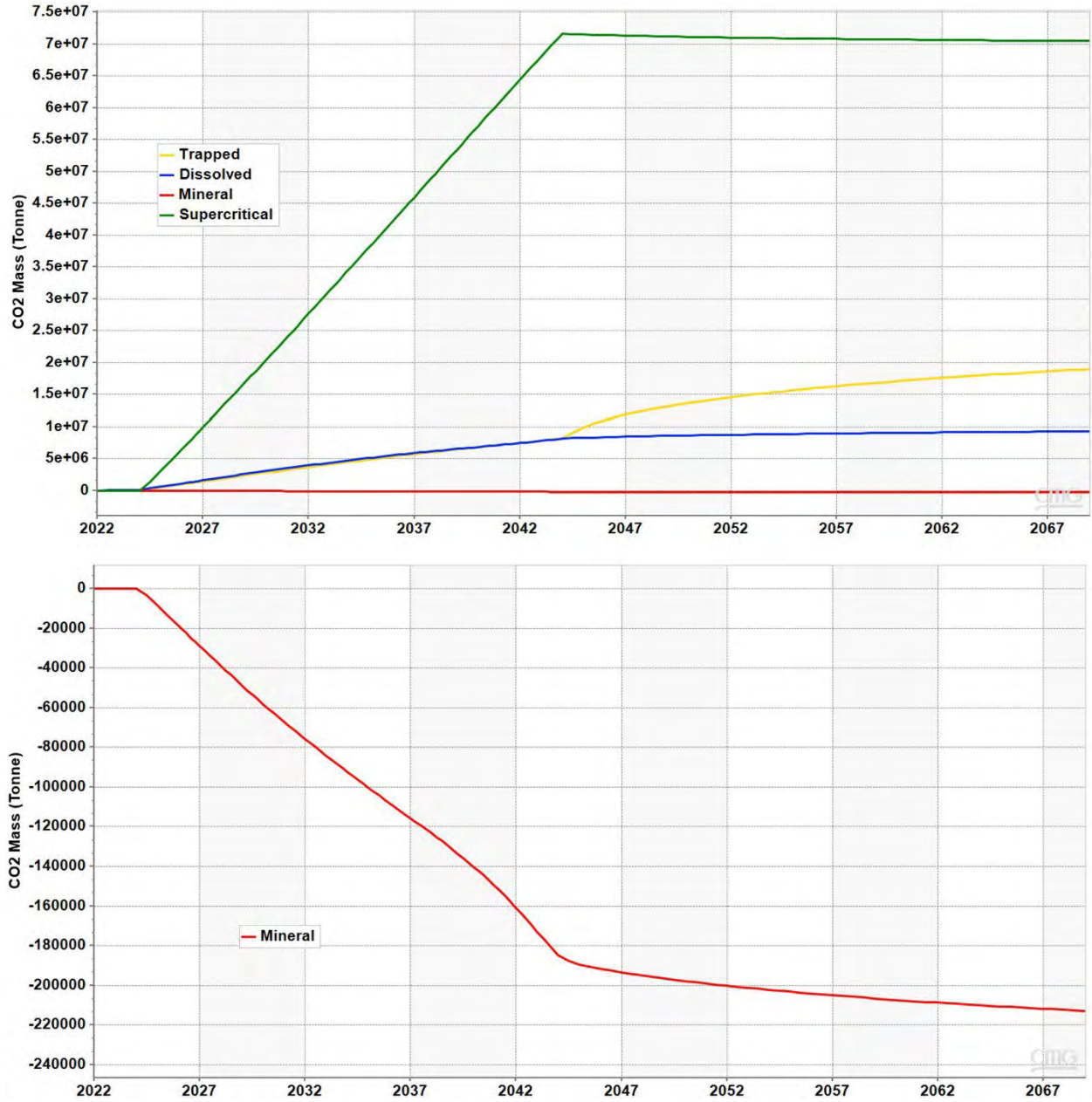
Figure C-8. Top image: mineral mass changes, in metric tons (tonnes), for the different CO 2 -trapping mechanisms present during CO 2 injection with geochemical modeling in the injection zone for the Broom Creek Formation; bottom image: CO 2 mineral trapping.
