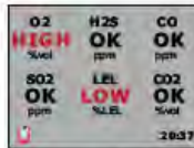
Alarms shown with "Go/No Go" text and flashing backlight.
