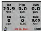
A "calibration due" warning appears for each relevant sensor.
