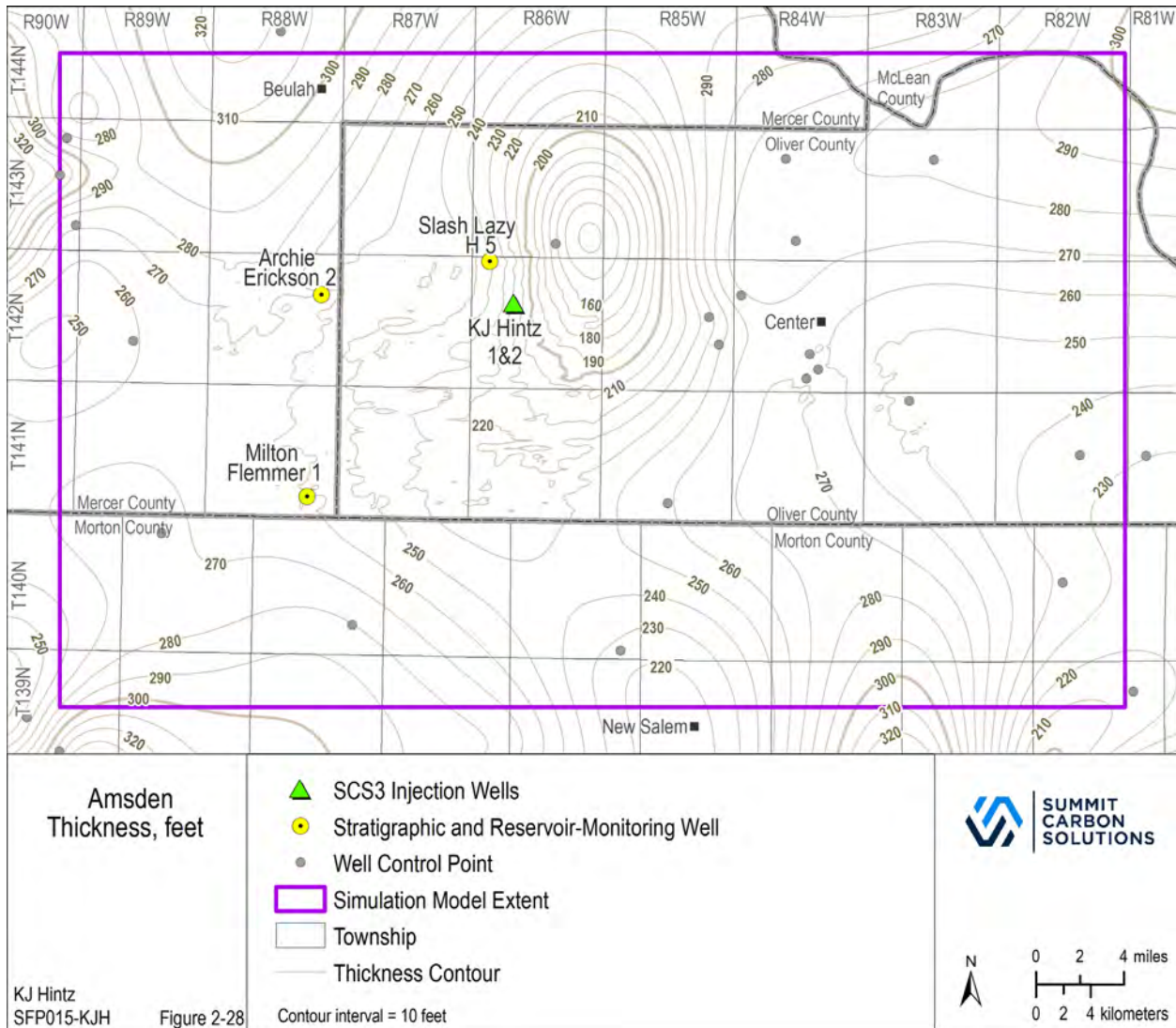
Figure 2-28. Isopach map of the Amsden Formation across the simulation model area. The convergent interpolation gridding algorithm was used with well formation tops, 3D seismic, and 2D seismic in creation of this map.
