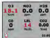
Bright red numerals and a flashing backlight show alarm conditions.
