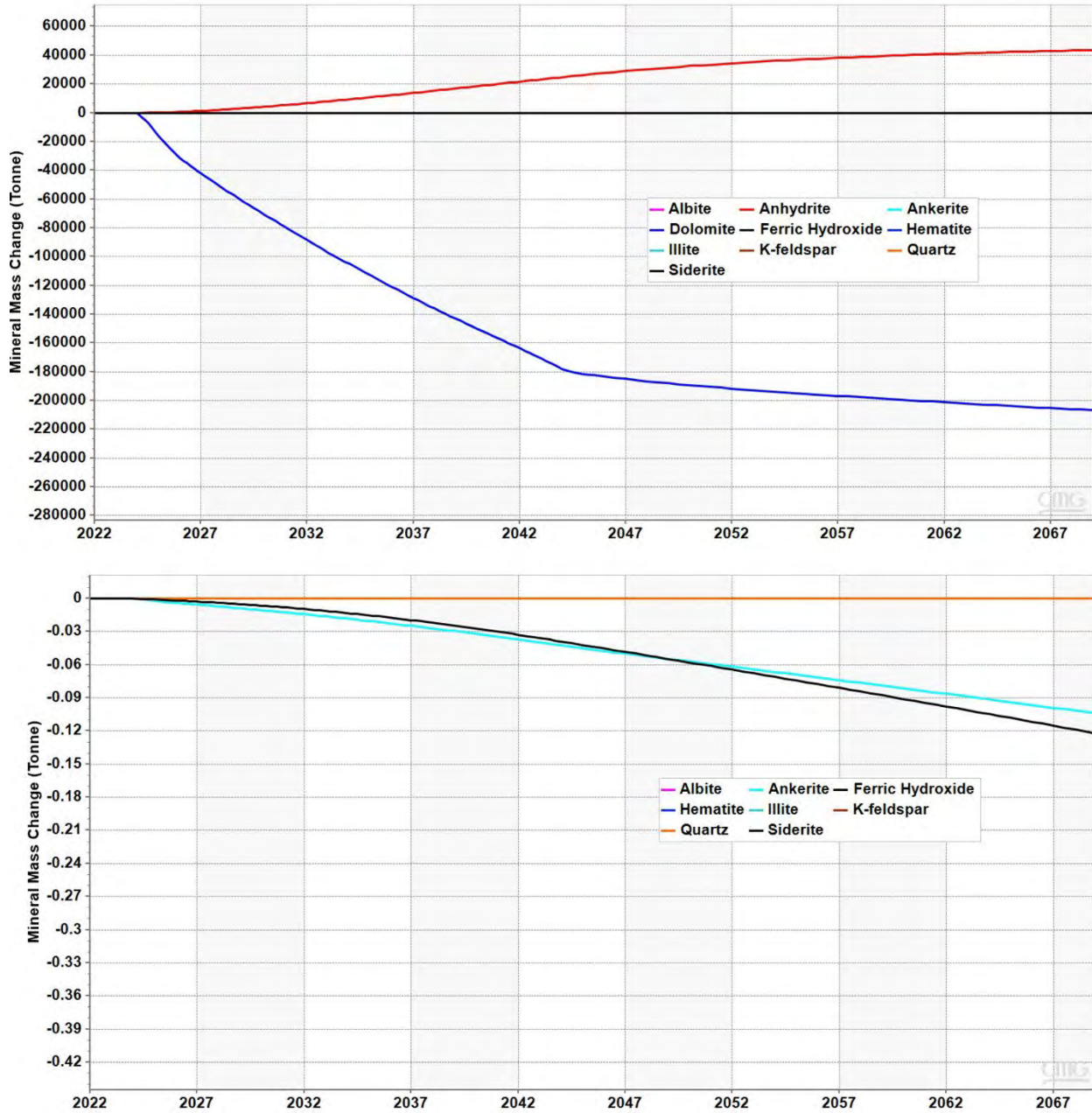
Figure C-7. Modeled change in the mineral masses (minus values show dissolution and positive values show precipitation) due to CO 2 injection (top: all minerals; bottom: zoomed-in after removing anhydrite and dolomite). Dissolution of dolomite with precipitation of anhydrite was observed. All of the other minerals showed very small values and account as net zero in this figure.
