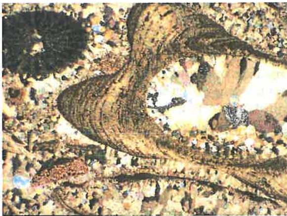
Figure A-5: Limestone With Fossil Fragments, Viewed under Crossed Polarizers.
