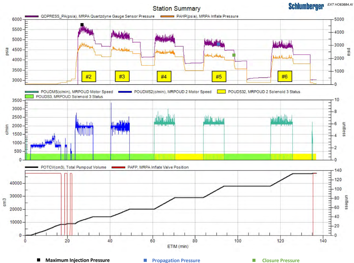
Figure 2-7. Milton Flemmer 1, Opeche/Spearfish Formation MDT microfracture in situ stress pump cycle graph at 5770.99 ft MD. No clear breakdown was observed.
