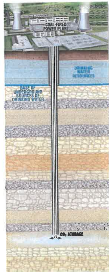
Class VI well schematic.
