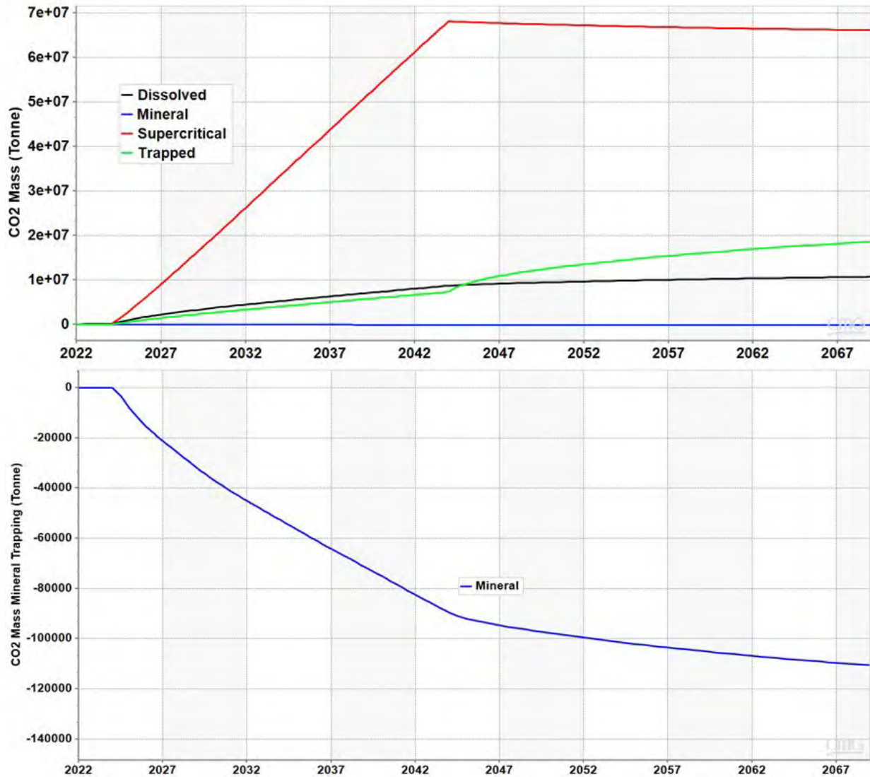
Figure C-8. Top image: mineral mass changes, in metric tons (tonnes), for the different CO 2 -trapping mechanisms present during CO 2 injection with geochemical modeling in the injection zone for the Broom Creek Formation; bottom image: CO 2 mineral trapping.
