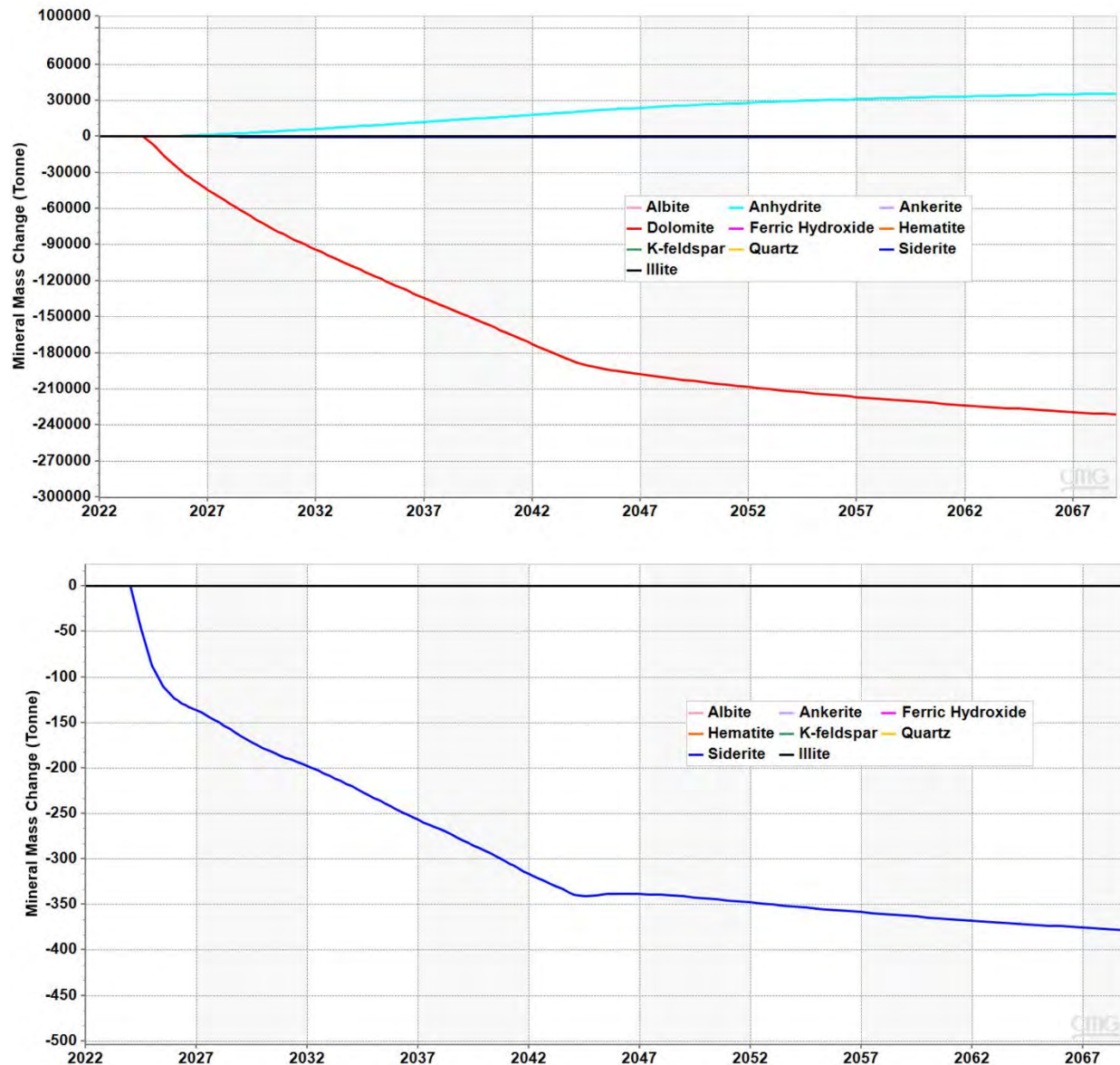
Figure C-7. Modeled change in the mineral masses (minus values show dissolution and positive values show precipitation) due to CO 2 injection (top: all minerals; bottom: zoomed in after removing anhydrite and dolomite). Dissolution of dolomite with precipitation of anhydrite was observed. All of the other minerals showed very small values and account as net zero in this figure.
