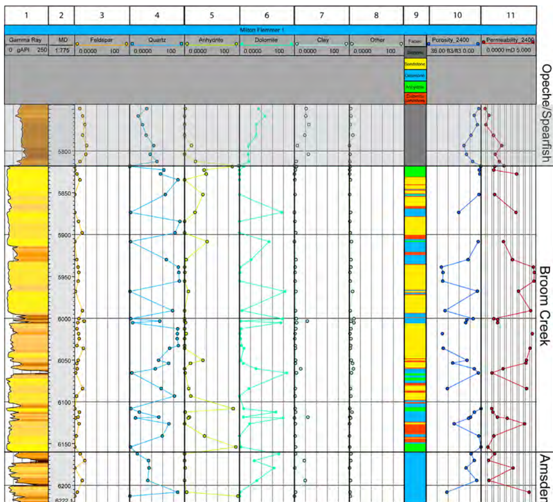
Figure 2-24. Change in the mineralogy of the upper-confining Opeche/Spearfish Formation (highlighted in gray) at Milton Flemmer 1 as a function of depth based on XRD in comparison to GR, facies, core sample total porosity (%), and permeability (mD). Very low total porosity and permeability with a high clay content make the Opeche/Spearfish Formation an ultralow permeable formation. Data gaps in the porosity and permeability plots are due to the inability to obtain testable samples as solid plugs (i.e., samples too soft/brittle). Tracks from left to right are 1) GR (black), 2) MD, 3) total feldspar (orange), 4) quartz (blue), 5) anhydrite (yellow green), 6) dolomite (green), 7) total clay (light blue), 8) other (light green), 9) facies, 10) core porosity (2400 psi) (dark blue), and 11) core permeability (2400 psi) (red).
