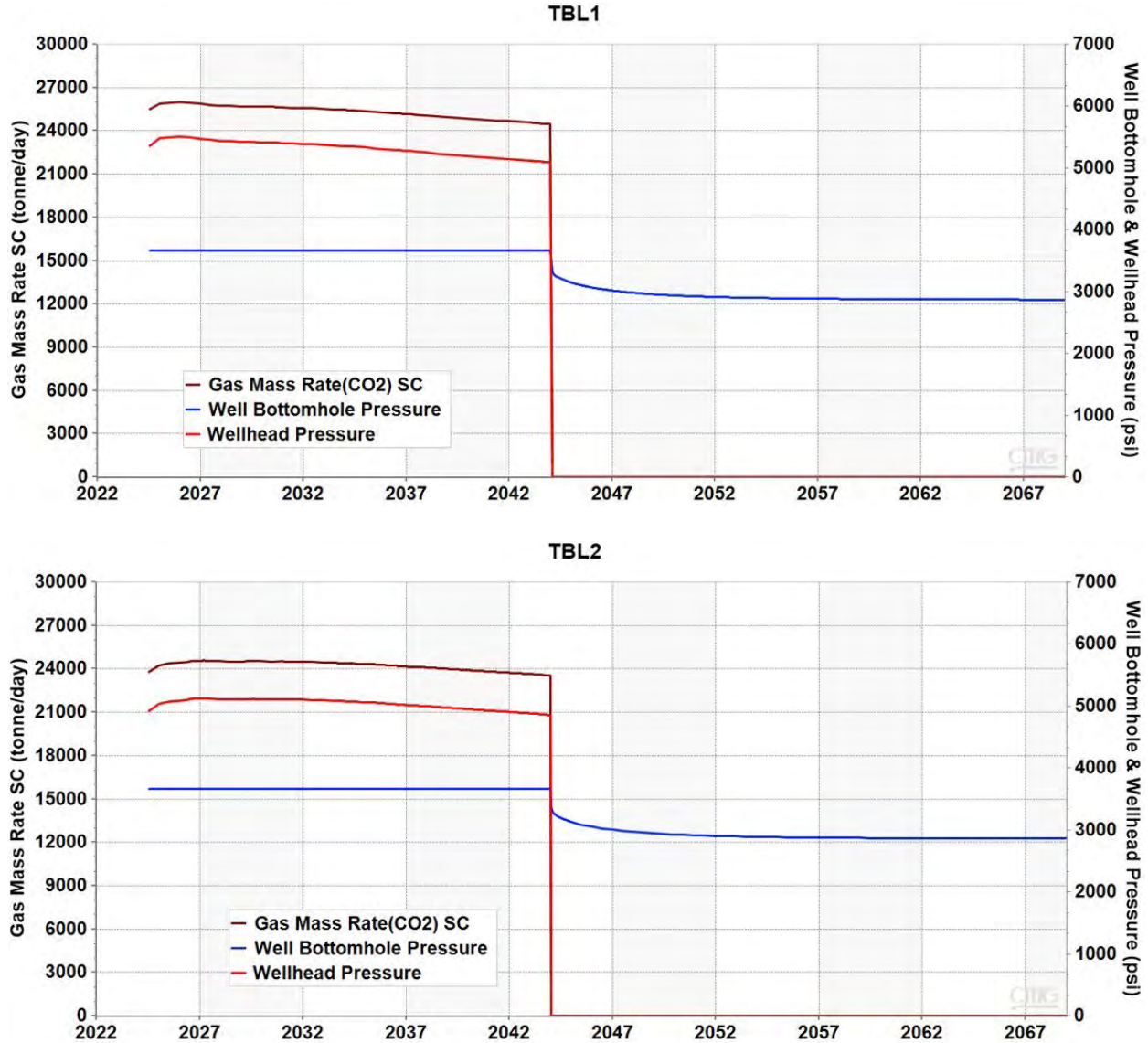
Figure 3-16. Maximum pressure and gas rate response when the well was operated at max BHP only (without any WHP limits) for TB Leingang 1 (top) and TB Leingang 2 (bottom).
