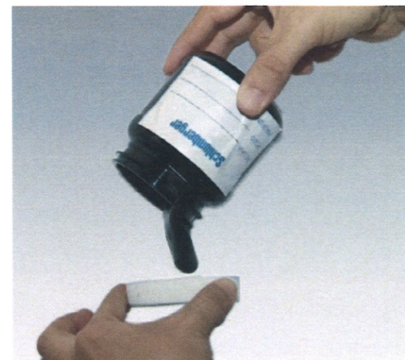
The Saturn 3D radial probe collected an uncontaminated sample of 7.5-API oil from an unconsolidated sandstone reservoir without sanding or seal failure.
