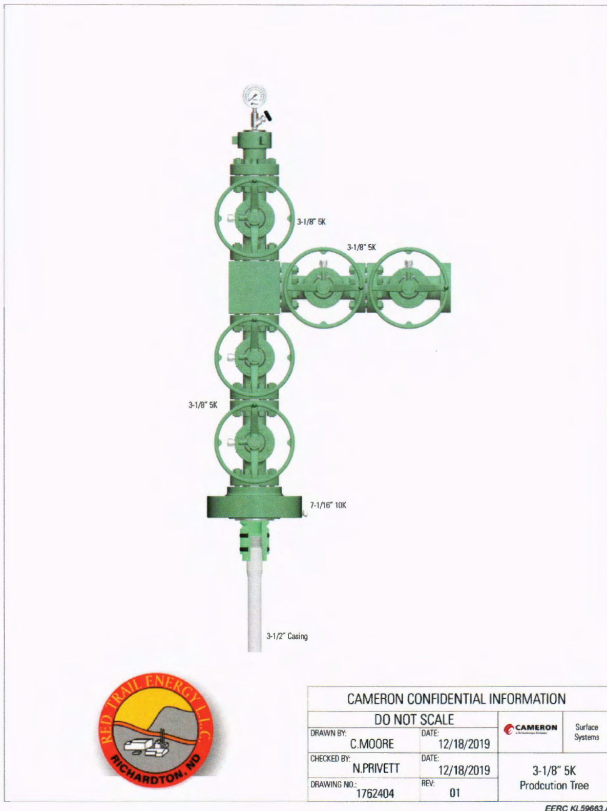
Figure 5-3. RTE-10 well – proposed CO 2 -resistant wellhead schematic – Cameron Supplier.
