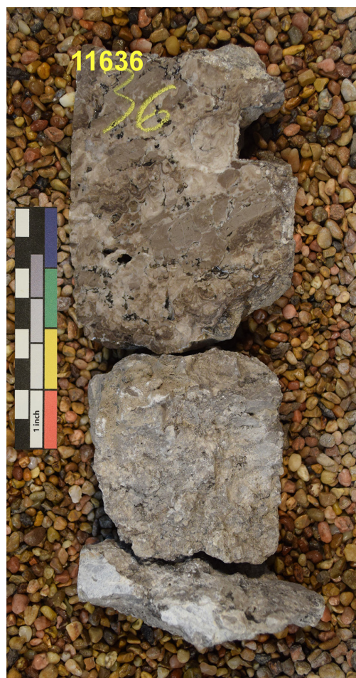
FIGURE 1. Core photo of Clarence Iverson #1 well core at 11,636 feet MD showing the pore space that produced the oil identified on April 4, 1951. Core stored in the Wilson M. Laird Core Library in Grand Forks, ND.
