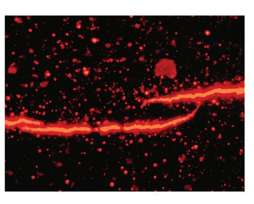
"Cracked\_tip" morphology of horizontal microfractures with widths of 10 to 20 microns. (Carlisle et. al., 1992).
