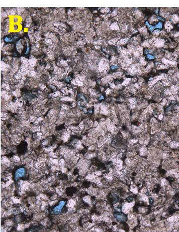
Balcron Oil – 44-24 Vaira (SESE Sec. 24, T24N, R54E) – Depth 10,011.0 ft. – Plane light photomicrographs of the reservoir consisting of a quartz dolostone with minor amounts of feldspars and clay. Intergranular porosity ranges from 10 -13%. A. 4X; B. 10X.
